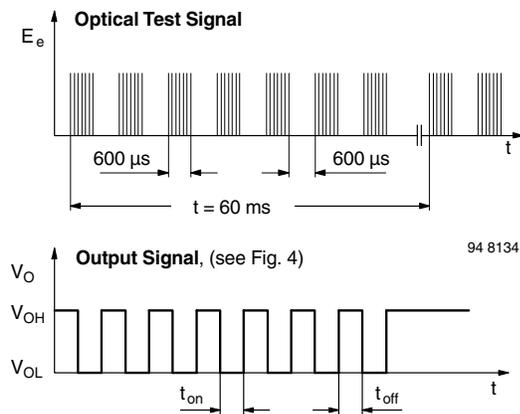
Fig. 3 - Test Signal
