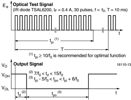
Fig. 1 - Output Delay and Pulse Width
