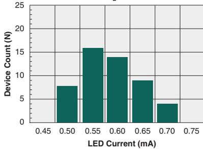
**Typical  $I_F$  For Switch Dropout**
