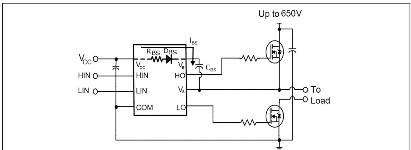
**Figure 13** Half bridge bootstrap circuit in 2ED218x
