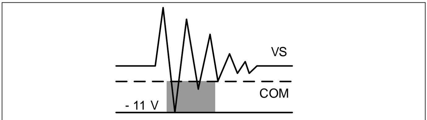
**Figure 19** Headroom for HV level shifter data transmission
