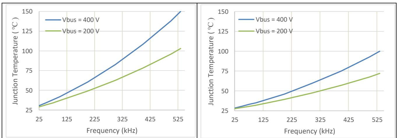
\*Assumptions for above curves: LLC topology, Power switch = IPP60R600P6,  $T_a = 25\text{ °C}$ ,  $V_{BUS} = 400\text{ V}$ ,  $V_{CC} = 12\text{ V}$ ,  $R_{gon} = 3.9\ \Omega$ ,  $R_{goff} = 1\ \Omega$
