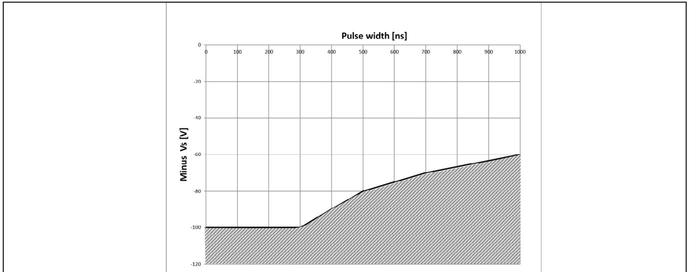
**Figure 18** Negative VS transient SOA for 2ED2106 (4) S06F (J) @  $V_{BS} = 15\text{ V}$
