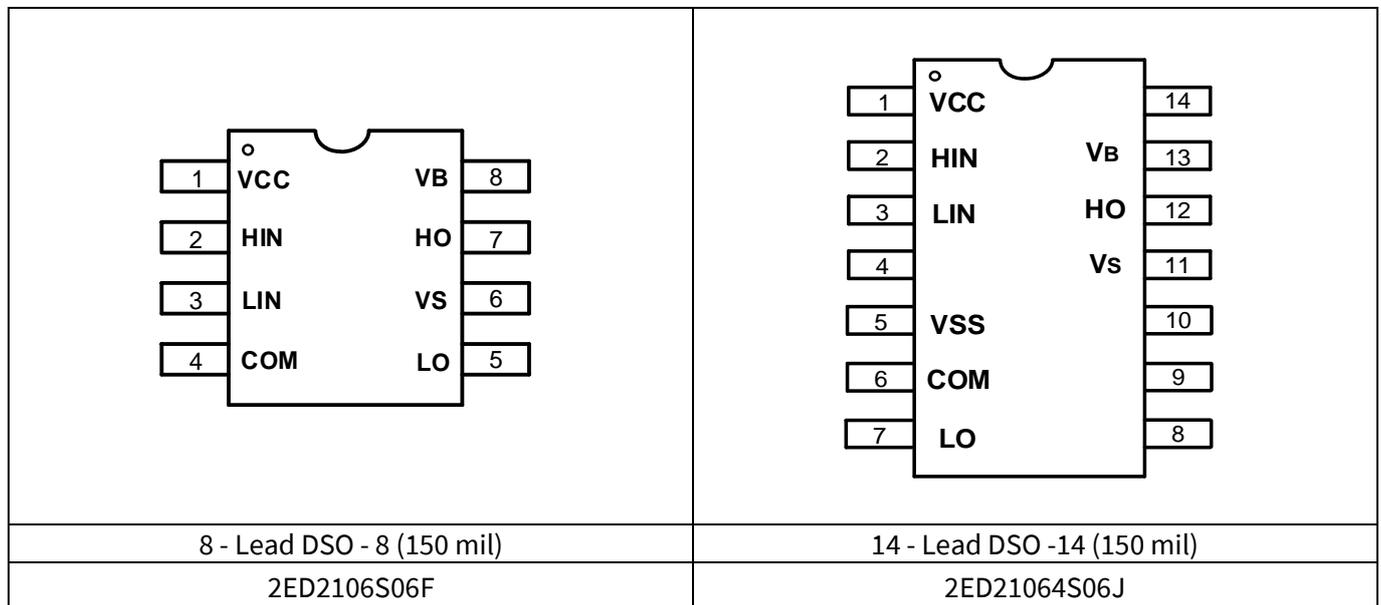
Figure 3 2ED2106(4)S06F(J) pin assignments (top view)
