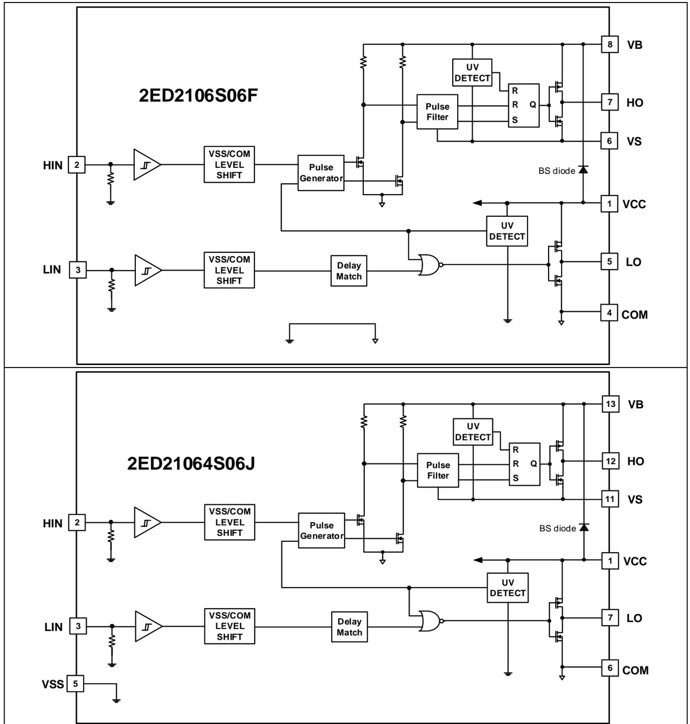
Figure 2 Block diagrams
