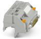
V8 adapter for 8 x PLC-INTERFACE (6.2 mm), controller: PLC system cabling of output cards, connection 1: Screw connection 1x, connection 2: D-SUB pin strip 1x 15-position, connection 3: Plug connection (Can be snapped onto 8x PLC-INTERFACE terminals), number of channels: 8, control logic: plusschaltend
