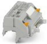
V8 adapter for 8 x PLC-INTERFACE (6.2 mm), controller: PLC system cabling of output cards, connection 1: Screw connection 1x, connection 2: IDC/FLK pin strip 1x 14-position, connection 3: Plug connection (Can be snapped onto 8x PLC-INTERFACE terminals), number of channels: 8, control logic: minusschaltend
