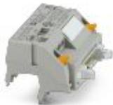
V8 adapter for 8 x PLC-INTERFACE (6.2 mm), controller: PLC system cabling of output cards, connection 1: Screw connection 1x, connection 2: IDC/FLK pin strip 1x 14-position, connection 3: Plug connection (Can be snapped onto 8x PLC-INTERFACE terminals), number of channels: 8, control logic: plusschaltend
