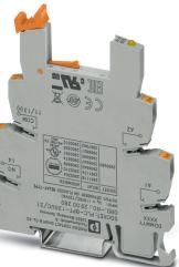
6.2 mm PLC basic terminal block with Push-in connection, without relay or solid-state relay, for mounting on DIN rail NS 35/7,5, 1 changeover contact, input voltage 120 V AC/DC
