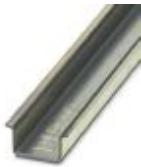
DIN rail, unperforated, Standard profile, width: 35 mm, height: 15 mm, similar to EN 60715, material: Steel, galvanized, passivated with a thick layer, length: 2000 mm, color: silver
