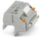
V8 adapter for 8 x PLC-INTERFACE (6.2 mm), controller: PLC system cabling of output cards, connection 1: Screw connection 1x, connection 2: D-SUB socket strip 1x 15-position, connection 3: Plug connection (Can be snapped onto 8x PLC-INTERFACE terminals), number of channels: 8, control logic: plusschaltend
