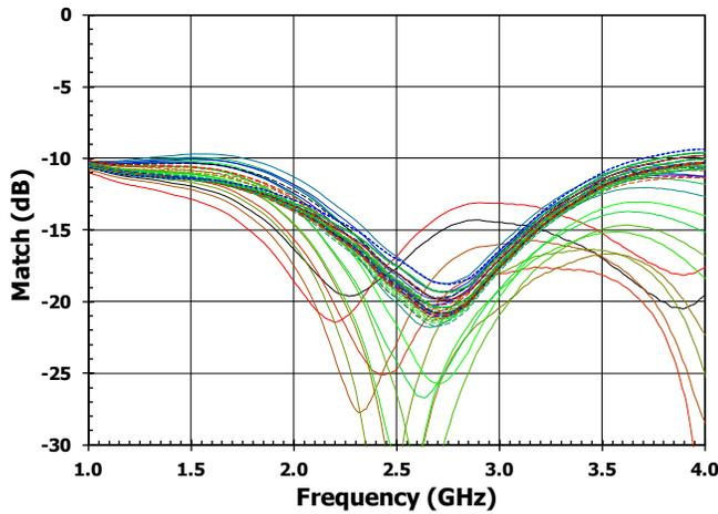
**Figure 17. Output Return Loss vs. Frequency**
