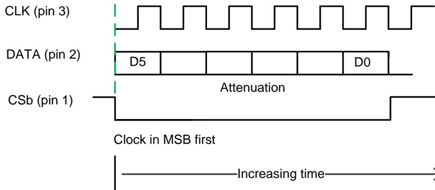
**Figure 53. SPI Timing Diagram**
