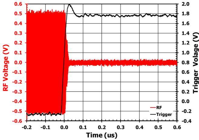
Figure 43. Switching Speed 31.5 to 0.0 dB
