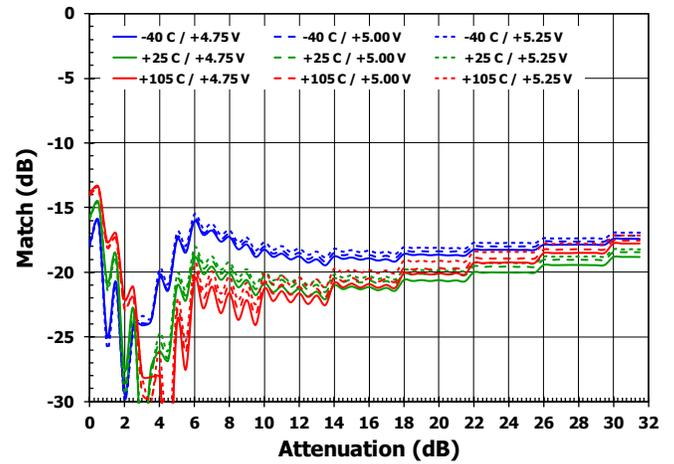
**Figure 18. Output Return Loss vs. Attenuation**
