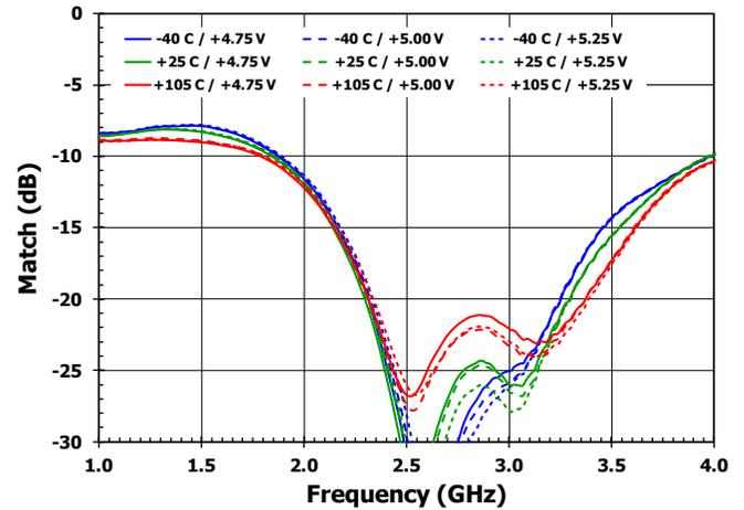
**Figure 8. EvKit Insertion Loss vs. Frequency over Temperature**
