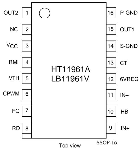
P-GND : Motor system ground
