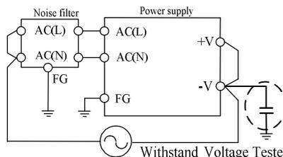
External capacitor adding point or short point. Even in the case of “+V and FG”, There is a similar effect.
