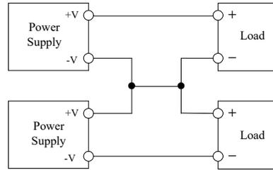
Note : In case of (A), please connect bypass diodes to prevent reverse voltage.
