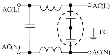
The example of noise filter circuit that may increasing capacitance value between “Input and FG”
