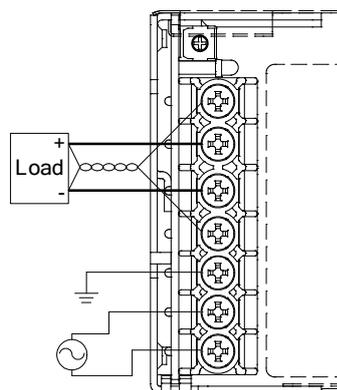
Recommended torque : HWS15A - HWS150A M3.5 screw 1.0N·m(10.2kgf·cm) - 1.6N·m(16.3kgf·cm)
