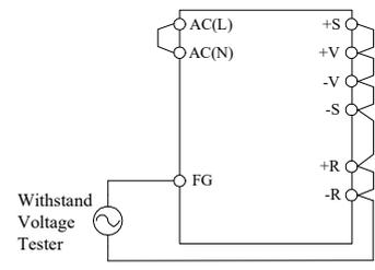
Note1 : This product have monolithic ceramic capacitor in secondary circuit to frame ground.
