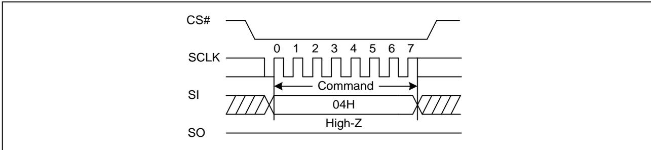
**Figure5a. Write Disable Sequence Diagram (QPI)**
