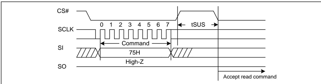
**Figure30a. Program/Erase Suspend Sequence Diagram (QPI)**
