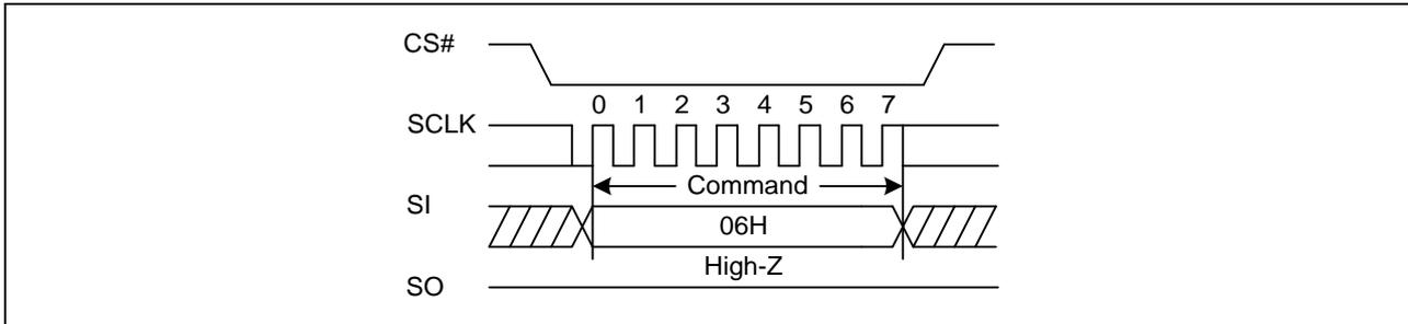
**Figure4a. Write Enable Sequence Diagram (QPI)**
