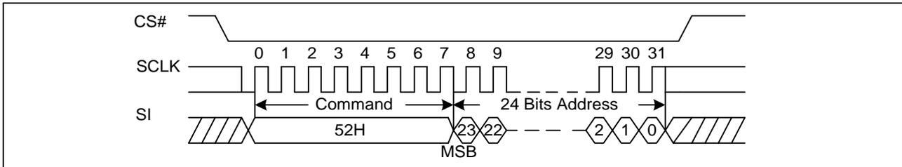
Note: The device default is in 24-bit address mode. For 4-byte mode, the address length becomes 32-bit.
