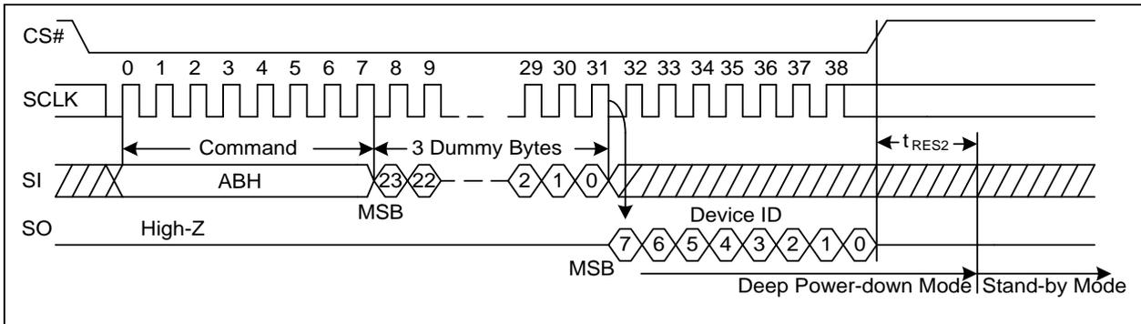
Figure25a. Release Power-Down/Read Device ID Sequence Diagram (QPI)
