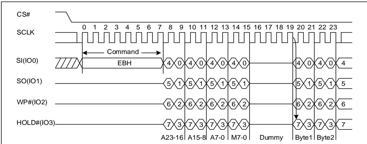
Note: The device default is in 24-bit address mode. For 4-byte mode, the address length becomes 32-bit.
