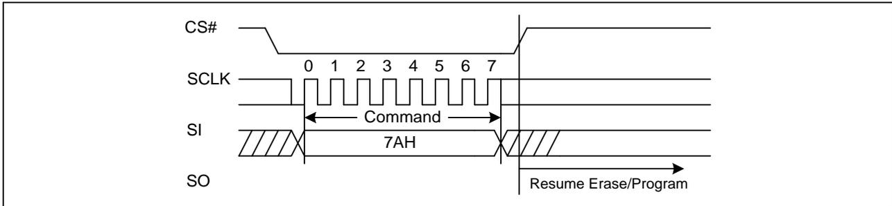
**Figure31a. Program/Erase Resume Sequence Diagram (QPI)**
