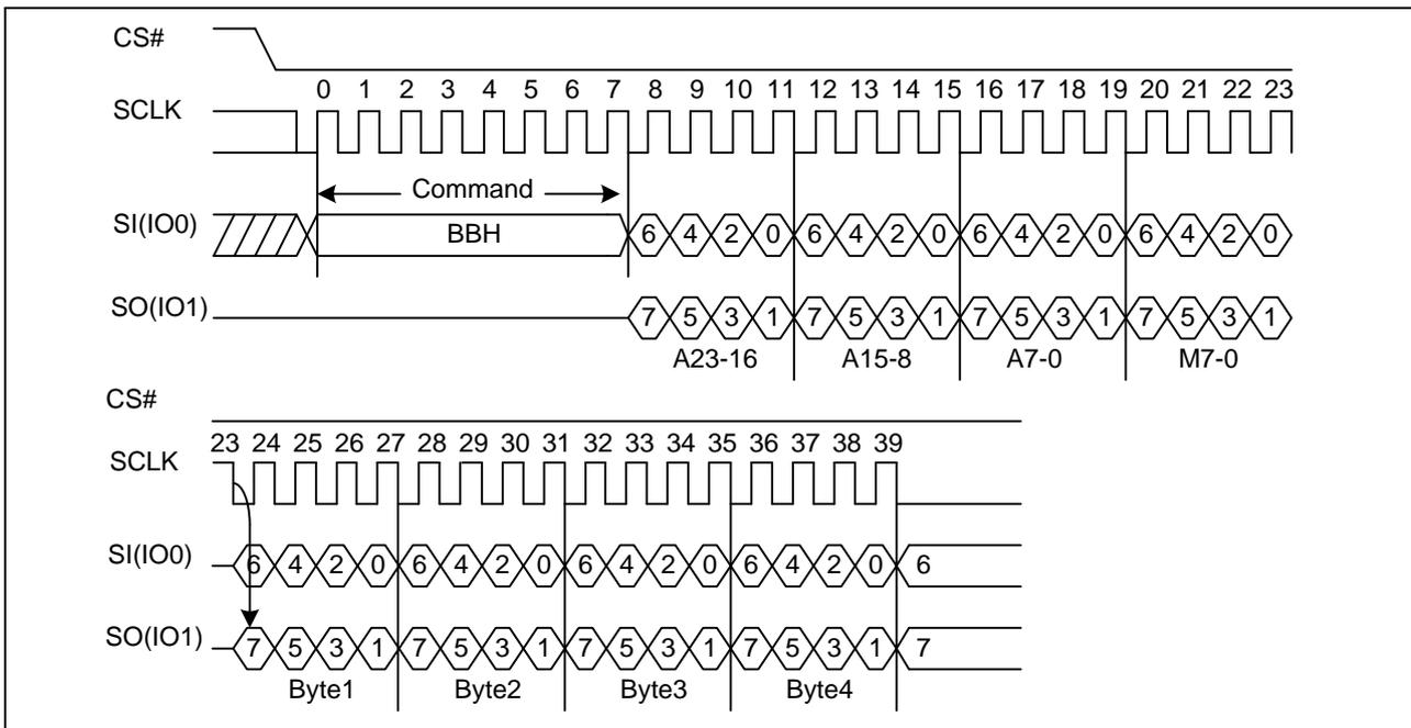
Note: The device default is in 24-bit address mode. For 4-byte mode, the address length becomes 32-bit.
