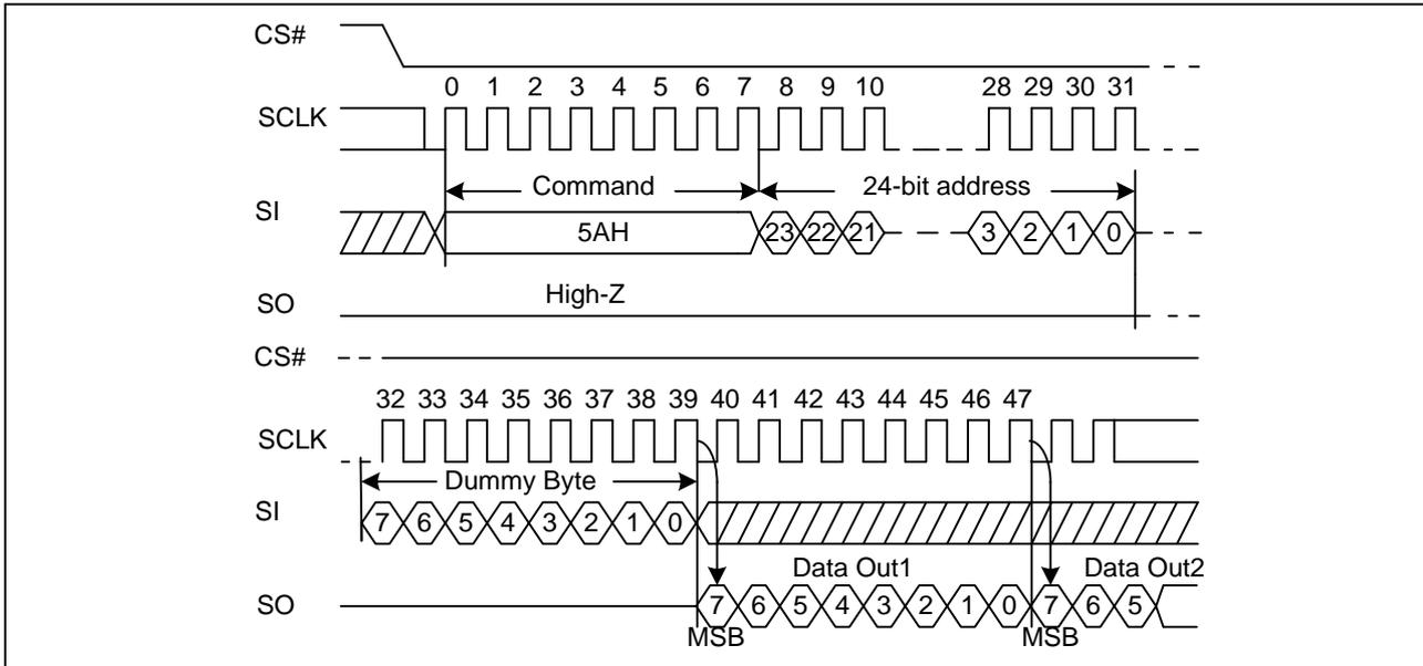
**Figure43a. Read Serial Flash Discoverable Parameter command Sequence Diagram (QPI)**
