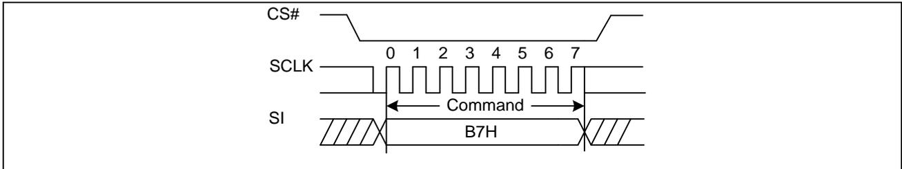
**Figure2a. Enable 4-byte Mode Sequence Diagram (QPI)**
