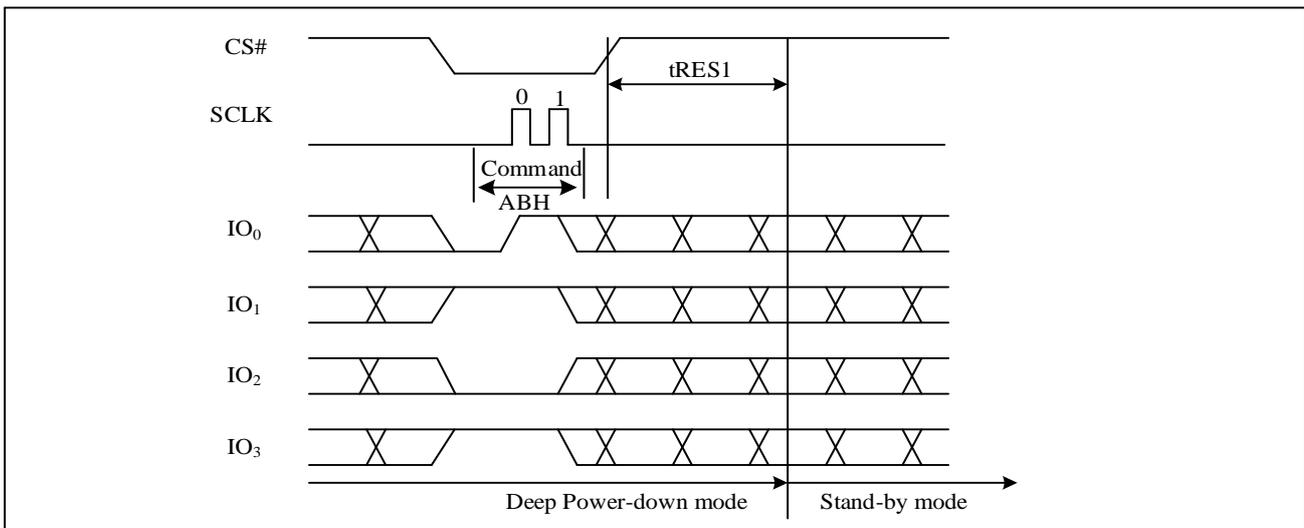
Figure25. Release Power-Down/Read Device ID Sequence Diagram
