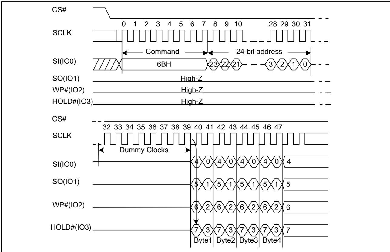
Note: The device default is in 24-bit address mode. For 4-byte mode, the address length becomes 32-bit.
