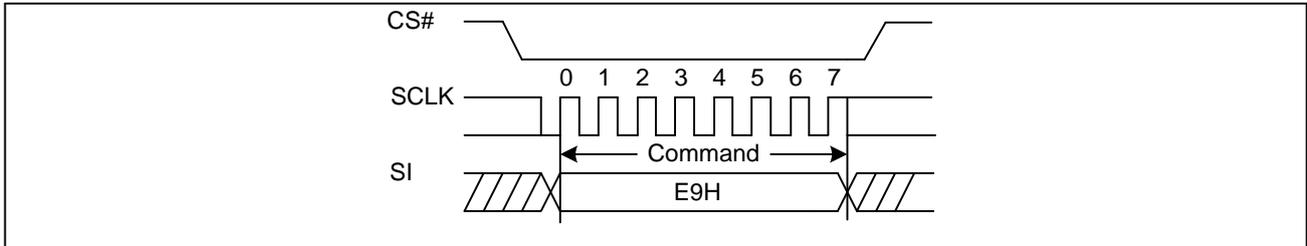
**Figure3a. Disable 4-byte Mode Sequence Diagram (QPI)**
