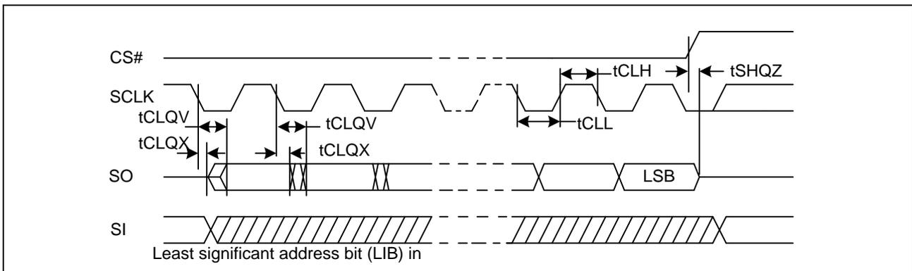
**Figure49. Resume to Suspend Timing Diagram**
