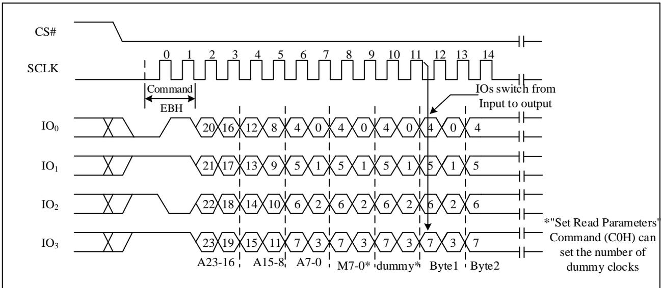
Note: The device default is in 24-bit address mode. For 4-byte mode, the address length becomes 32-bit.
