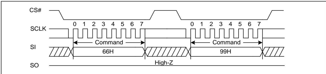
**Figure42a. Enable Reset and Reset command Sequence Diagram (QPI)**
