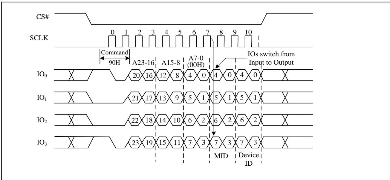
**7.25. Read Manufacture ID/ Device ID Dual I/O (92H)**
