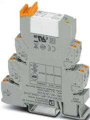
PLC-INTERFACE for high continuous currents, consisting of PLC-BPT.../21 HC basic terminal block with Push-in connection and plug-in miniature relay, for mounting on DIN rail NS 35/7,5, limiting continuous current up to 10 A, 1 changeover contact, input voltage 120 V AC/DC
