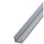
DIN rail, unperforated, Standard profile, width: 35 mm, height: 15 mm, similar to EN 60715, material: Aluminum, uncoated, length: 2000 mm, color: silver
