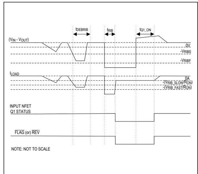
Figure 11. Fast Reverse Current Fault Timing Diagram
