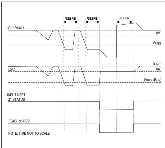
Figure 10. Slow Reverse Current Fault Timing Diagram
