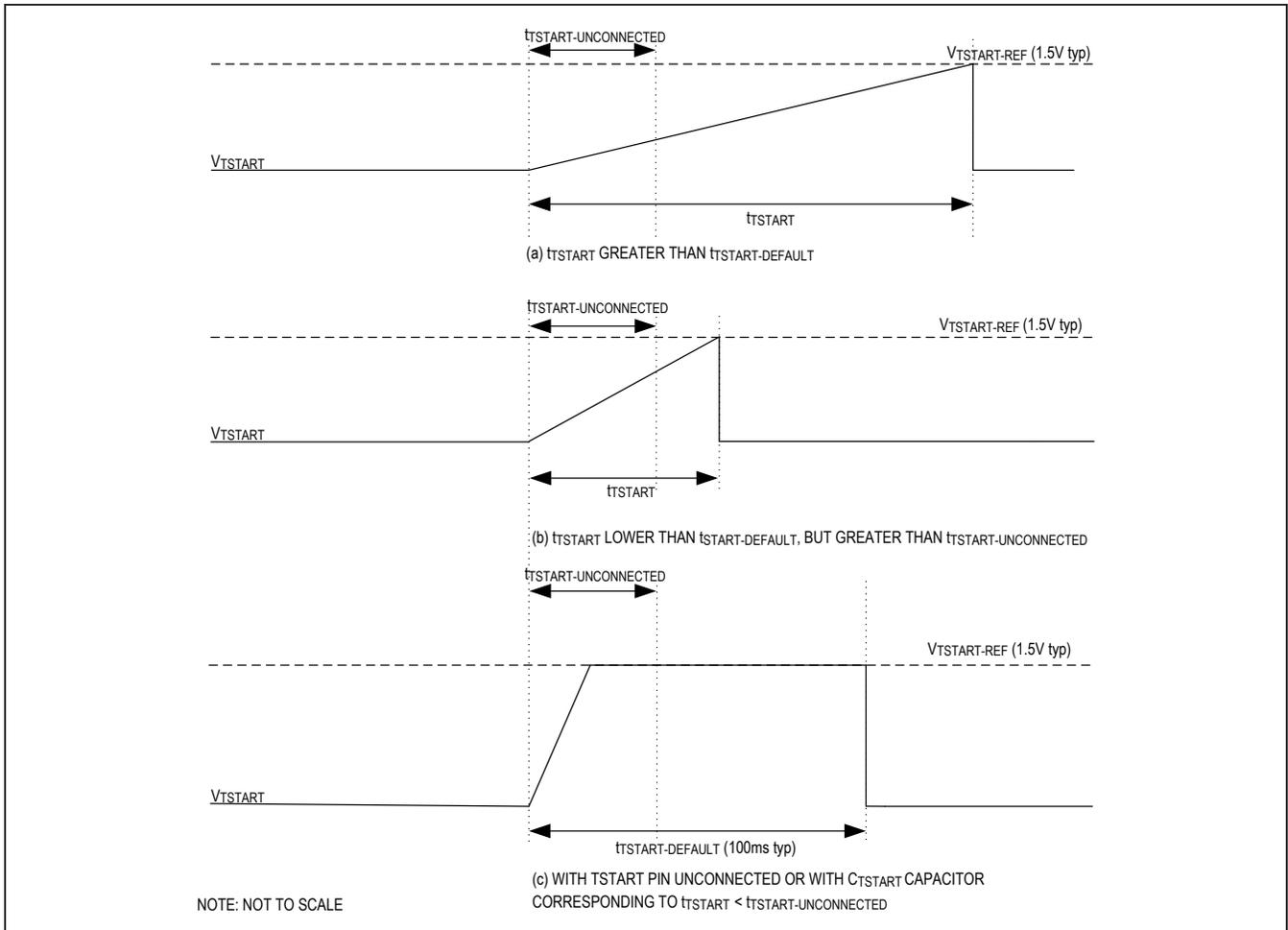
Figure 3. Startup Behavior with Respect to  $C_{TSTART}$
