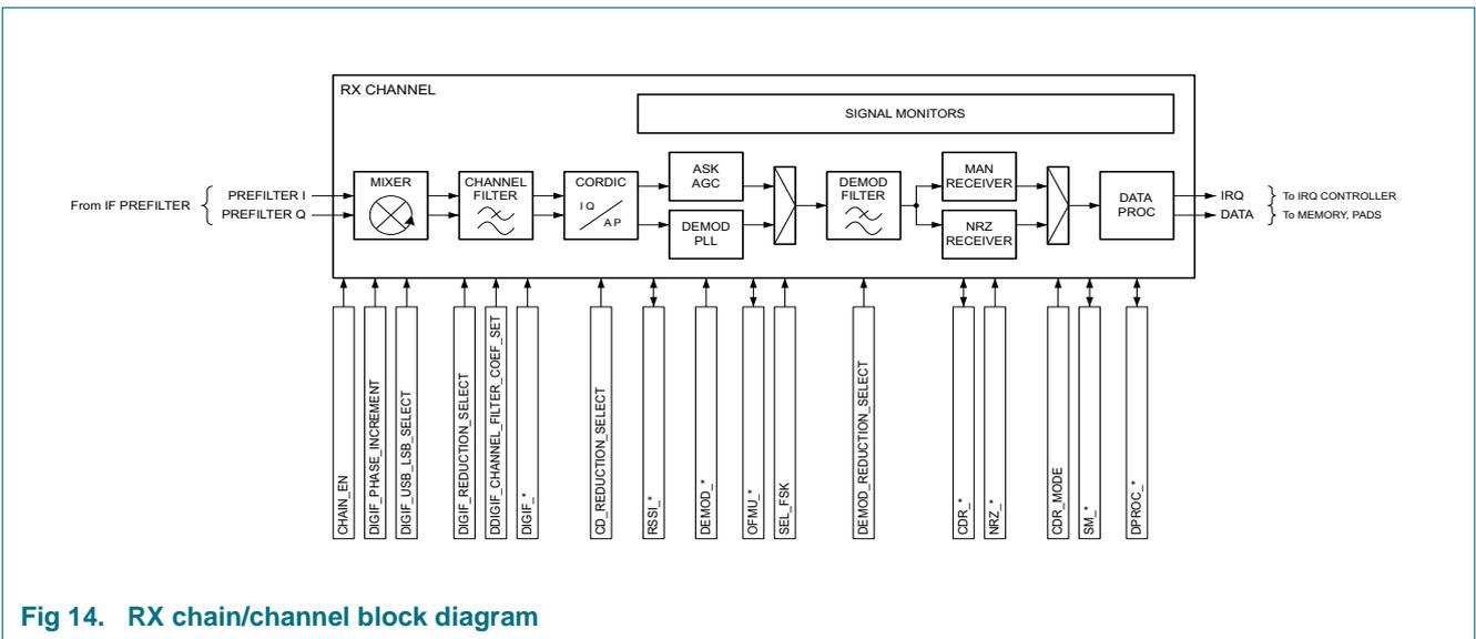
Fig 14. RX chain/channel block diagram
