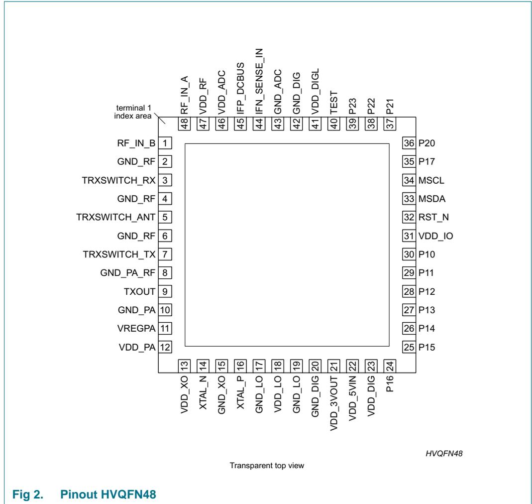
Fig 2. Pinout HVQFN48
