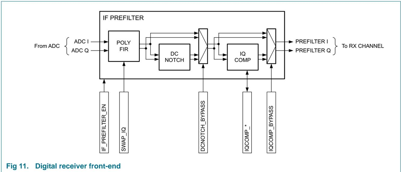
Fig 11. Digital receiver front-end
