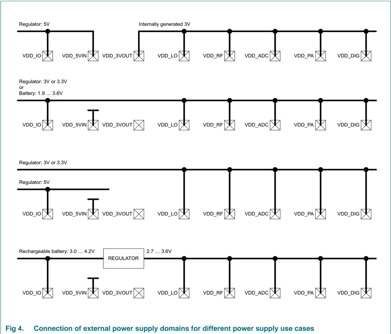
Fig 4. Connection of external power supply domains for different power supply use cases
