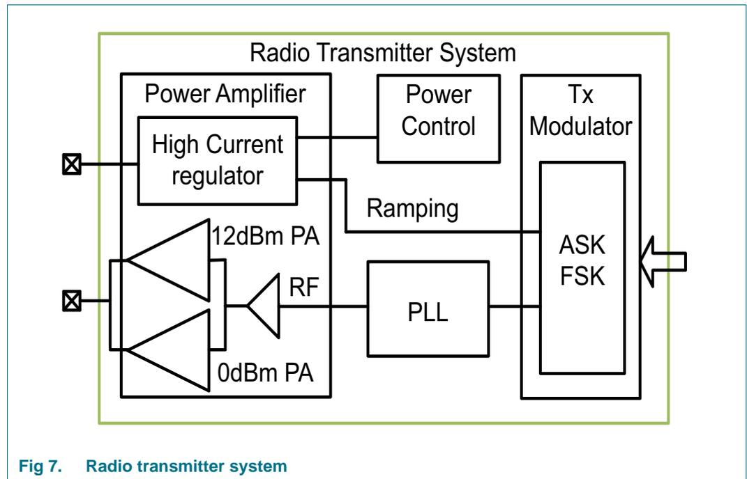
Fig 7. Radio transmitter system
