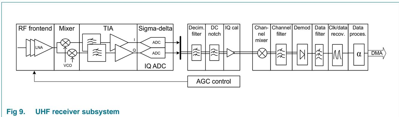
Fig 9. UHF receiver subsystem
