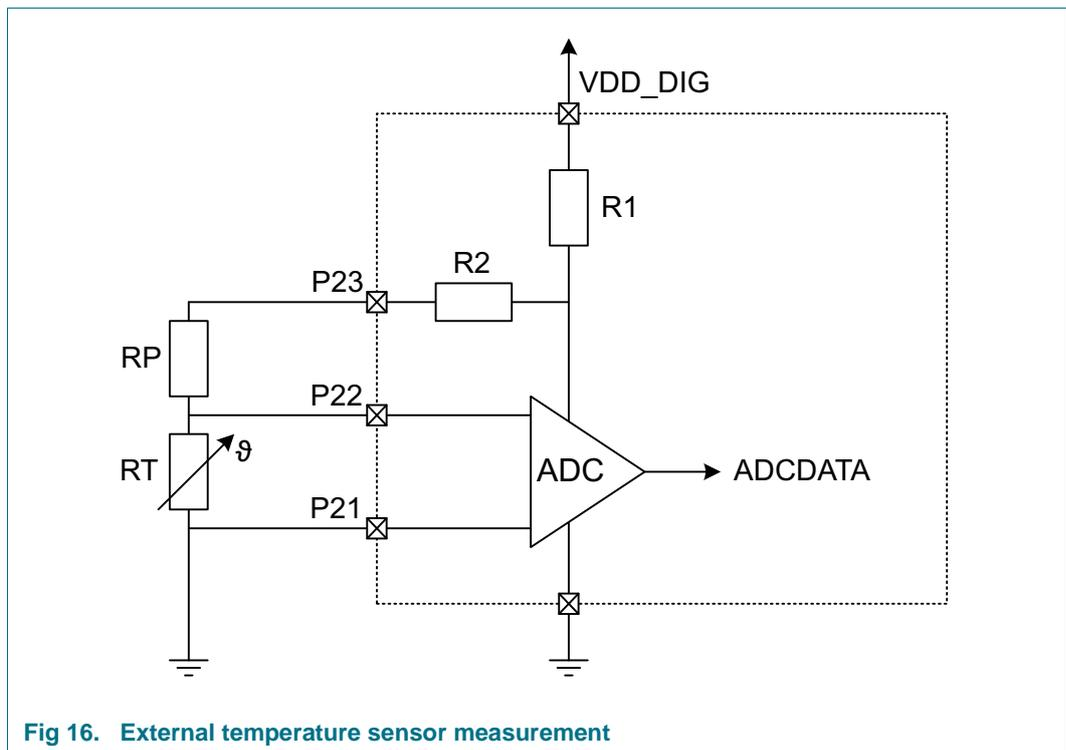
**Fig 16. External temperature sensor measurement**
