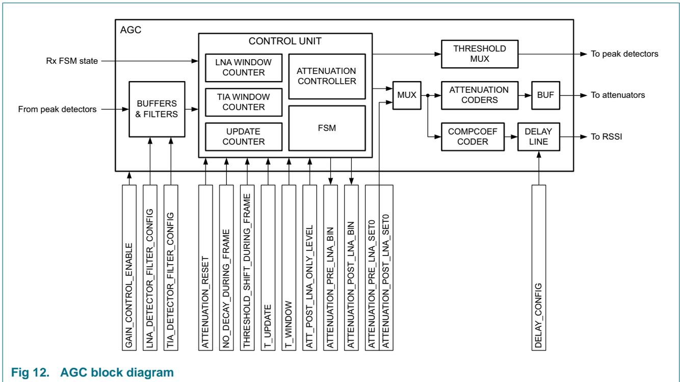
Fig 12. AGC block diagram
