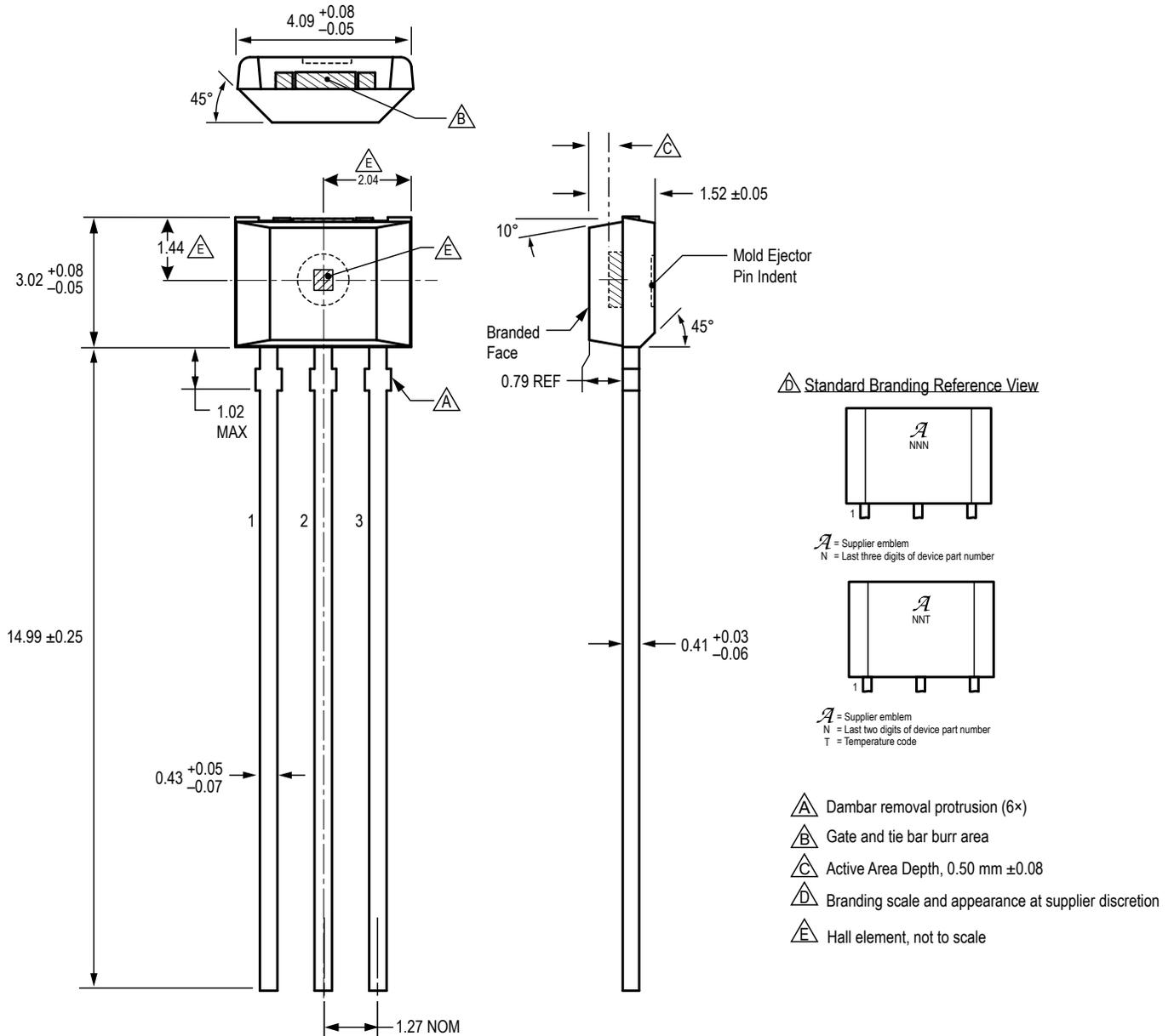
Figure 4: Package UA, 3-Pin SIP, Matrix Style
