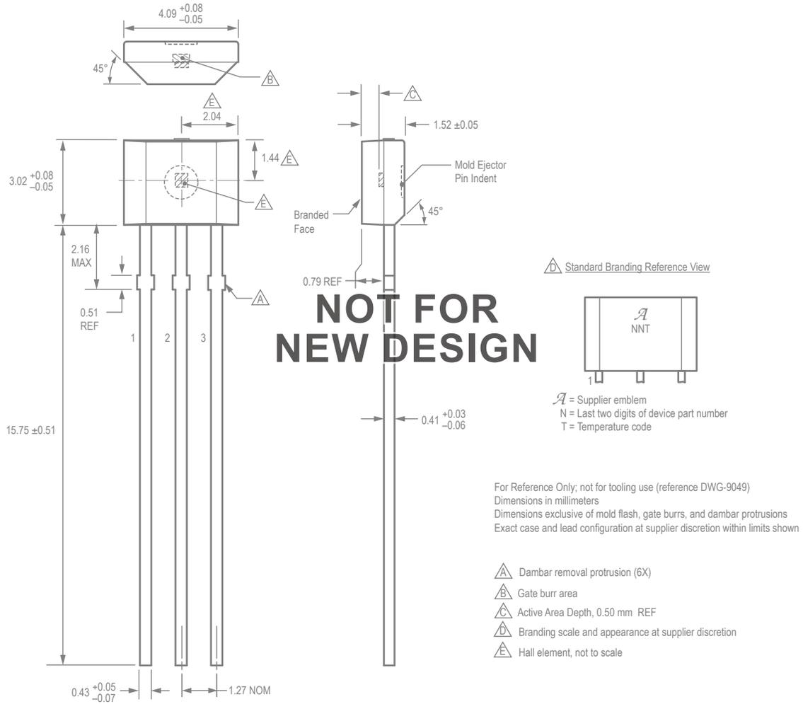
Figure 5: Package UA, 3-Pin SIP, Chopper Style
