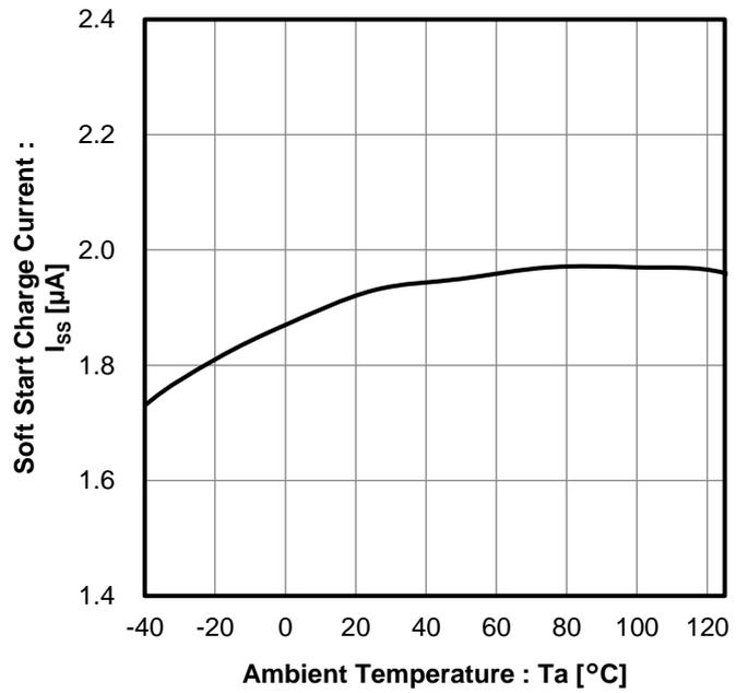
Figure 18. Soft Start Charge Current vs Ambient Temperature
