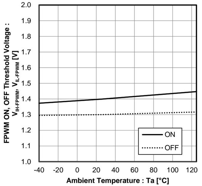
Figure 14. FPWM ON/OFF Threshold Voltage vs Ambient Temperature
