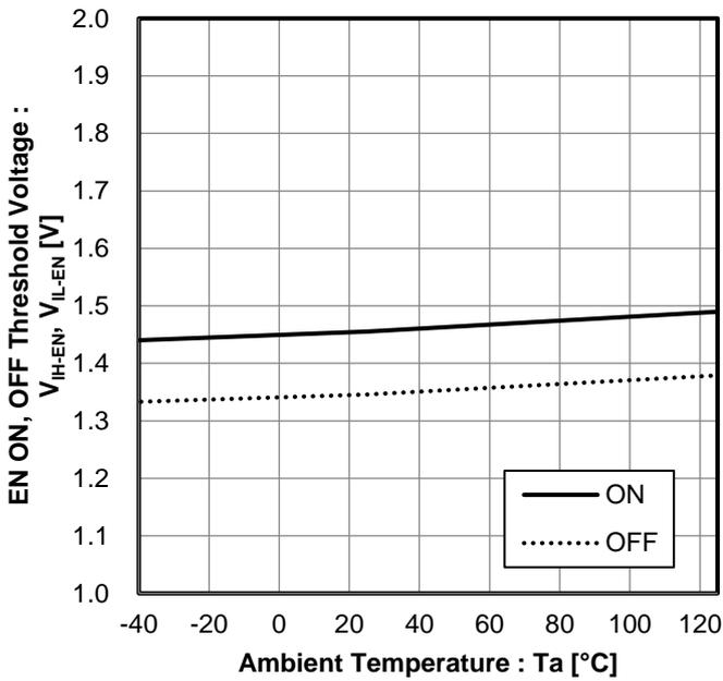
Figure 19. EN ON/OFF Threshold Voltage vs Ambient Temperature
