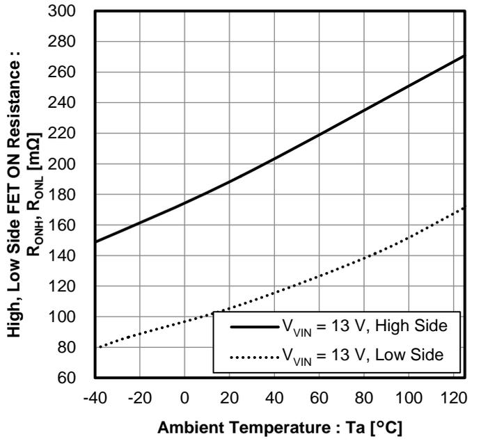
Figure 6. High/Low Side FET ON Resistance vs Ambient Temperature
