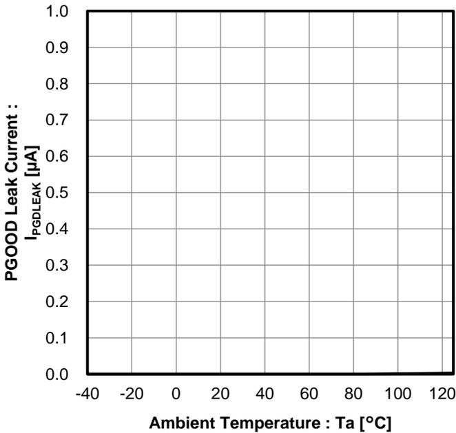
Figure 23. PGOOD Leak Current vs Ambient Temperature
