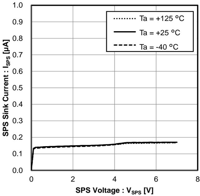
Figure 17. SPS Sink Current vs SPS Voltage
