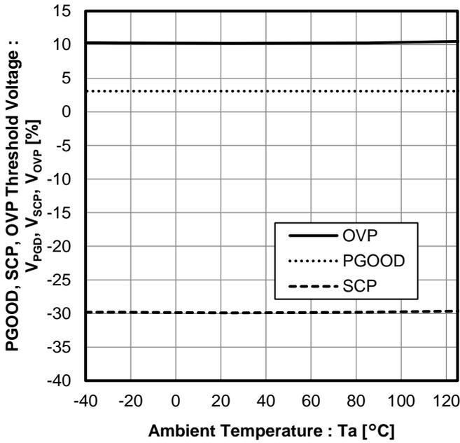
Figure 21. PGOOD/SCP/OVP Threshold Voltage vs Ambient Temperature
