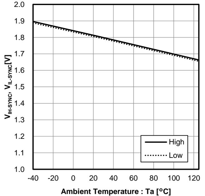
Figure 12. SYNC High/Low Threshold Voltage vs Ambient Temperature
