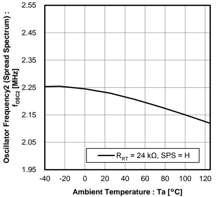
Figure 10. Oscillator Frequency2 (Spread Spectrum) vs Ambient Temperature
