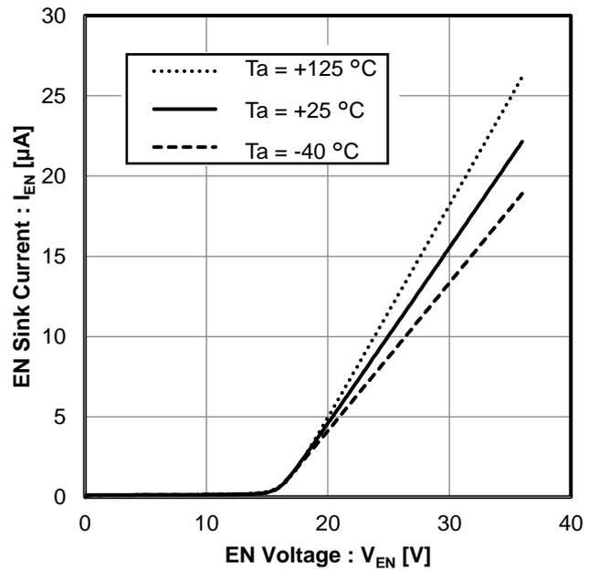
Figure 20. EN Sink Current vs EN Voltage
