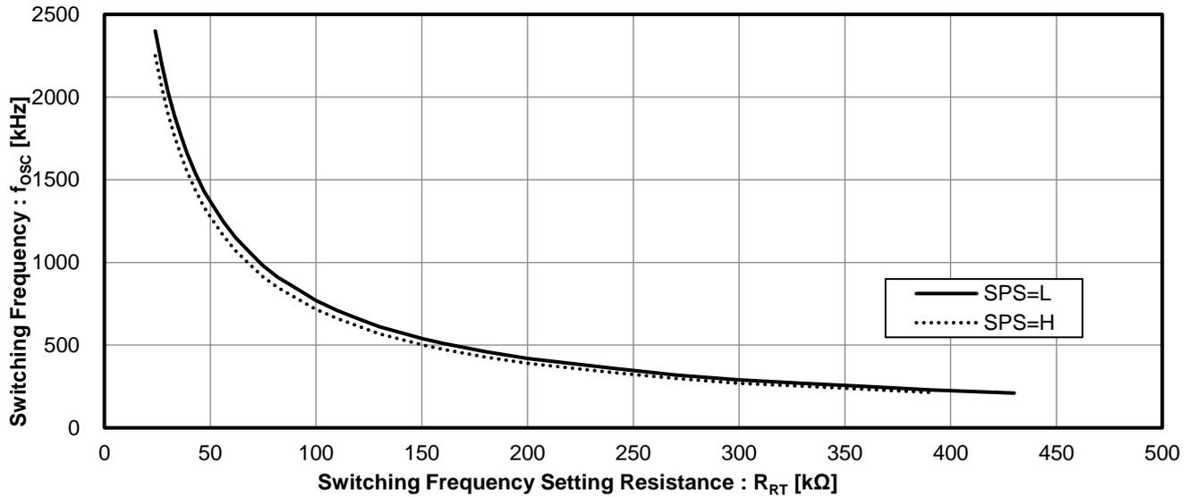
Figure 32. Switching Frequency vs Switching Frequency Setting Resistance
