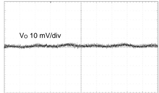
Figure 39. Output Ripple Voltage
