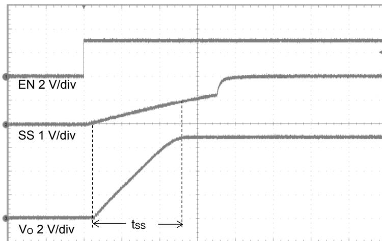
Figure 35. Soft start waveform
