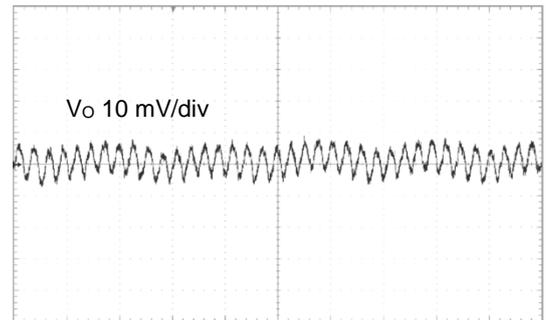
Figure 46. Output Ripple Voltage
