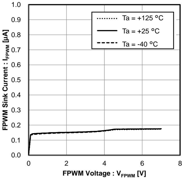
Figure 15. FPWM Sink Current vs FPWM Voltage
