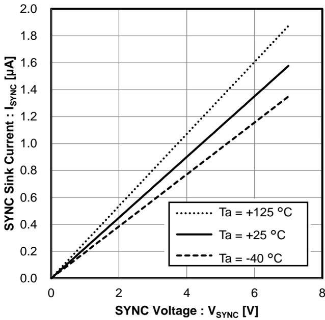
Figure 13. SYNC Sink Current vs SYNC Voltage
