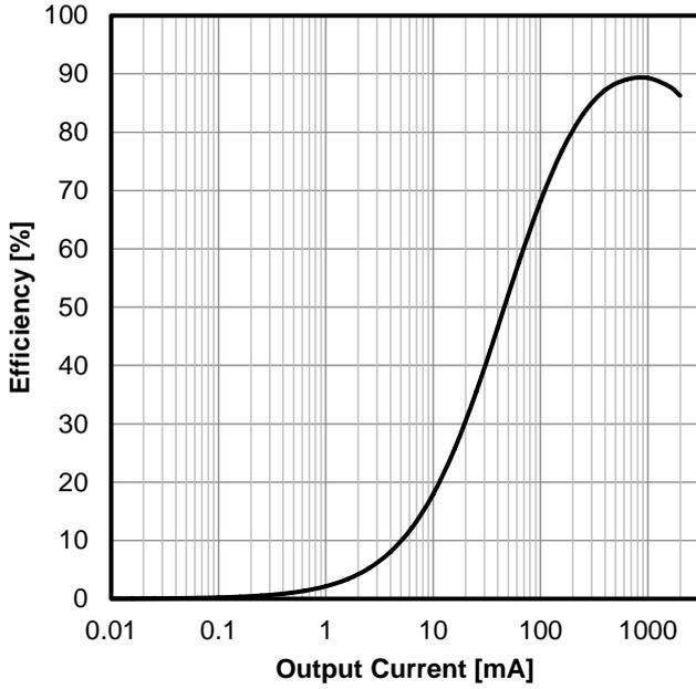
Figure 43. Efficiency vs Output Current
