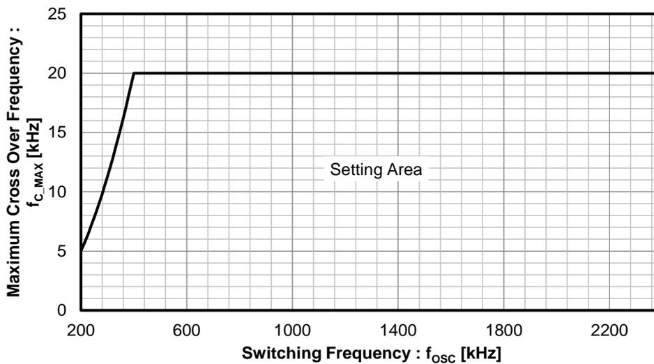
Figure 34. Maximum Cross Over Frequency vs Switching Frequency
