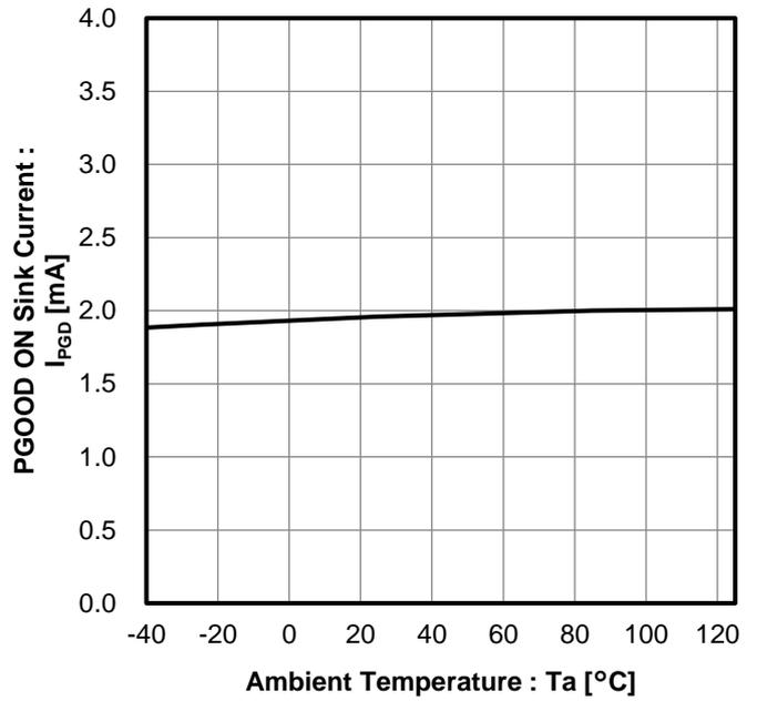
Figure 22. PGOOD ON Sink Current vs Ambient Temperature
