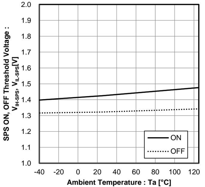
Figure 16. SPS ON/OFF Threshold Voltage vs Ambient Temperature
