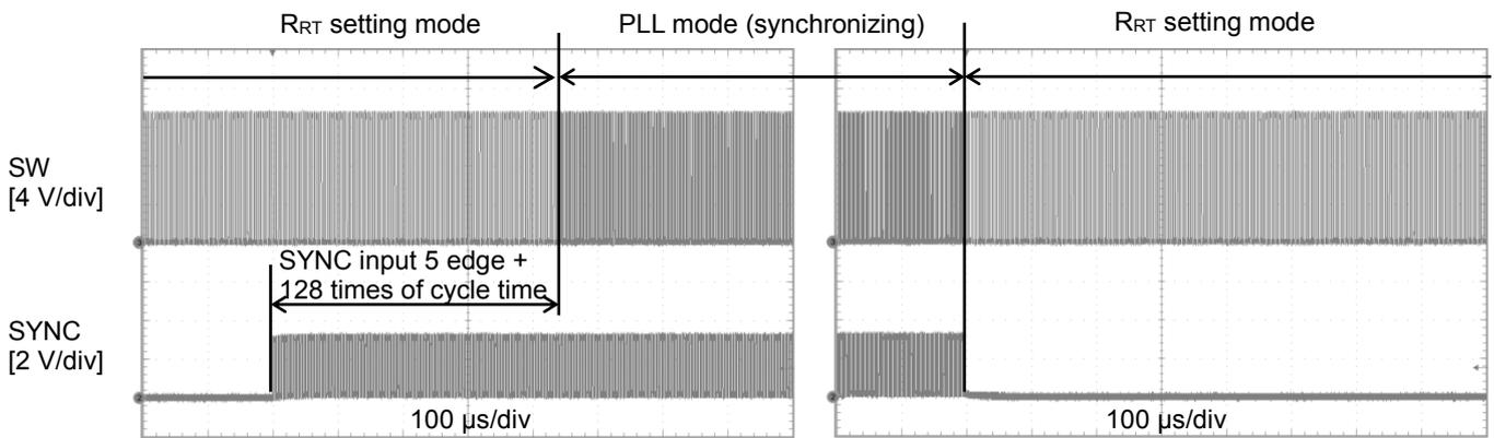
Figure 28. PLL OFF to ON waveform
