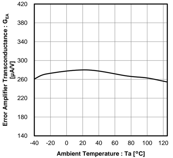
Figure 8. Error Amplifier Transconductance vs Ambient Temperature
