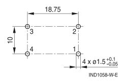
Tolerances to ISO 2768-cl / ISO 8015. Size ISO 14405 © All dimensions in mm
