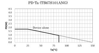
The power dissipation depends on the PCB layout and mounting conditions so please becareful. Also, when the ambient temperature is high, the allowed power disspation will be smaller.
