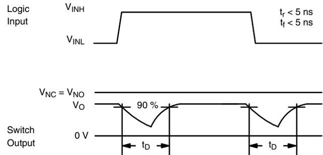
Fig. 2 - Break-Before-Make Interval
