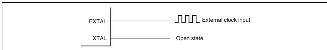
**Figure 4.4 Example of External Clock Connection**
