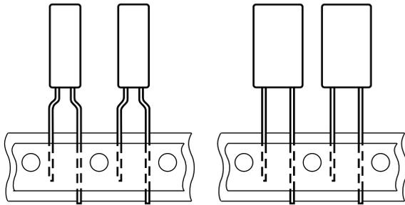
Case  $\varnothing D \times L = 5 \text{ mm} \times 11 \text{ mm}$  and  $8.2 \text{ mm} \times 11 \text{ mm}$
