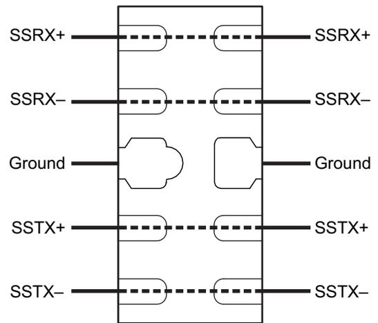
Figure 4. Flow Through Layout for USB 3.1
