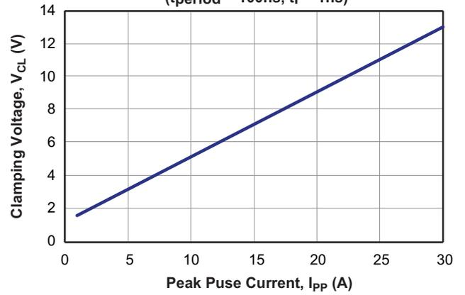
+8kV ESD Clamping Per IEC 61000-4-2
