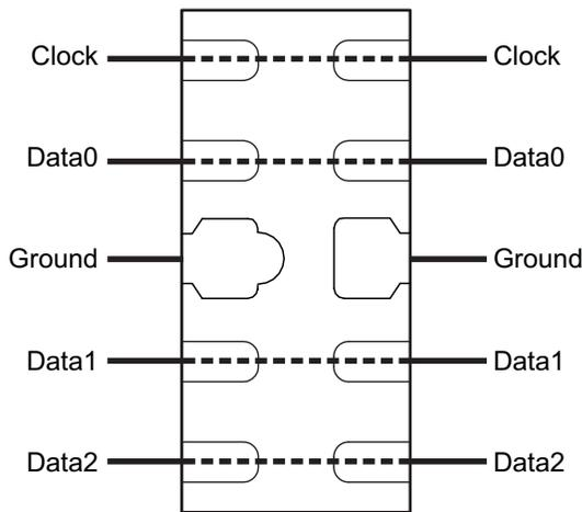
Figure 3. Flow Through Layout for HDMI 1.4/2.0
