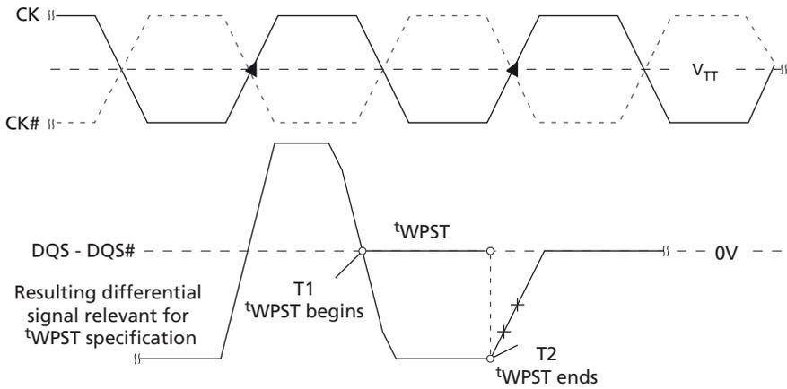
Figure 82: WRITE Burst
