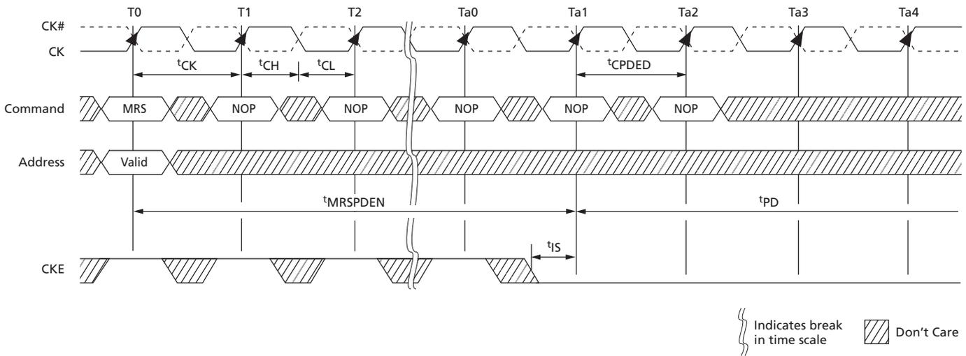
Figure 104: Power-Down Exit to Refresh to Power-Down Entry
