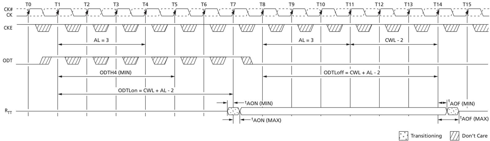
Note: 1.  $AL = 3$ ;  $CWL = 5$ ;  $ODTLon = WL = 6.0$ ;  $ODTLoff = WL - 2 = 6$ .  $R_{TT,nom}$  is enabled.
