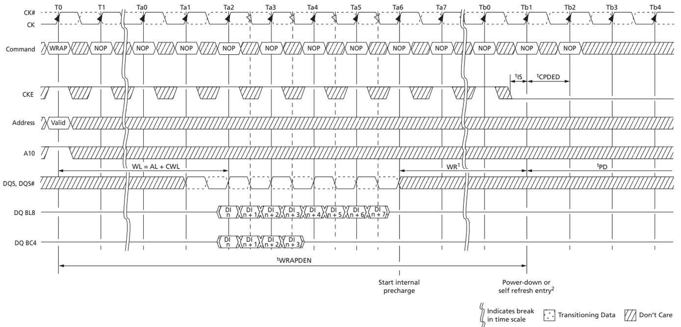
Notes: 1.  $t_{WR}$  is programmed through MR0[11:9] and represents  $t_{WRmin}$  (ns)/ $t_{CK}$  rounded up to the next integer  $t_{CK}$ .
