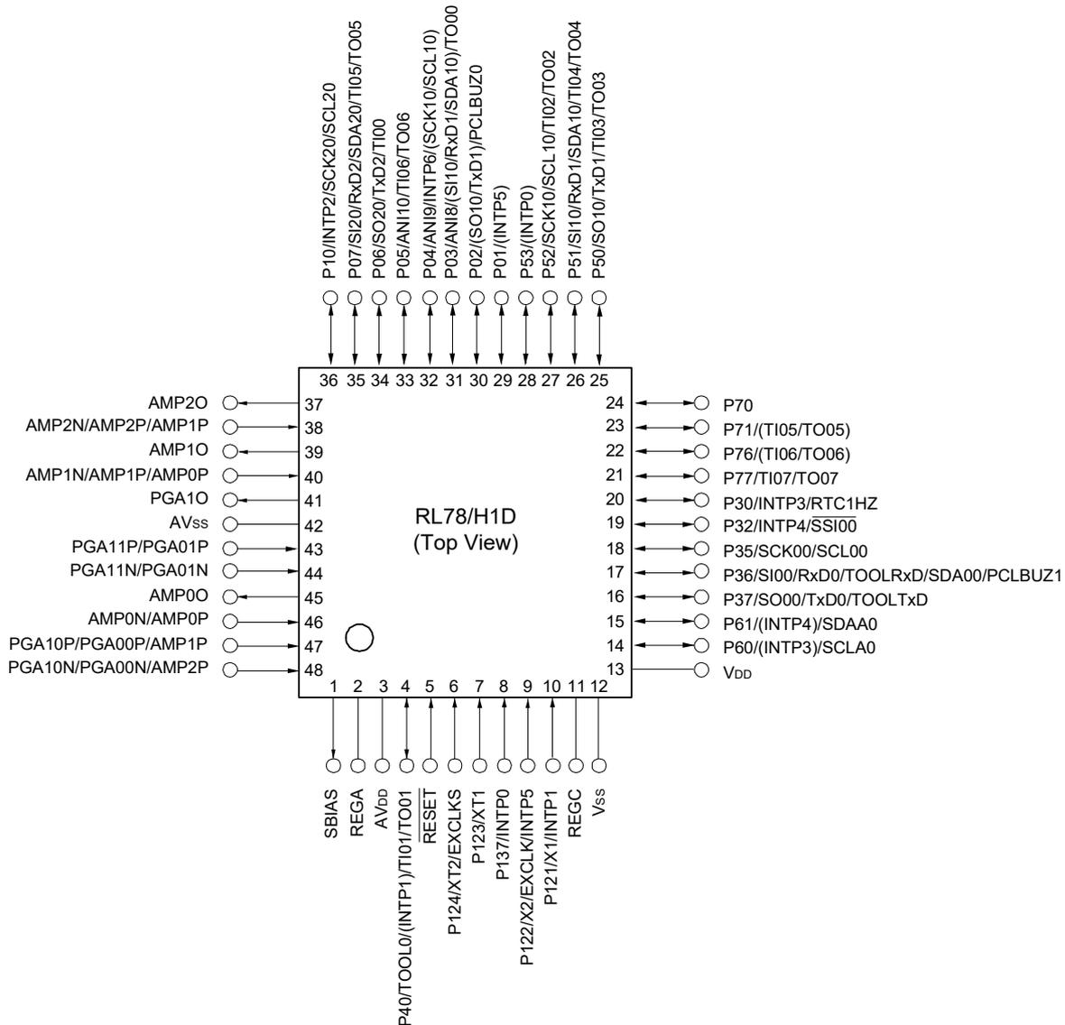
**Caution 1.** Connect the REGC pin to V<sub>SS</sub> pin via a capacitor (0.47 to 1 μF).
