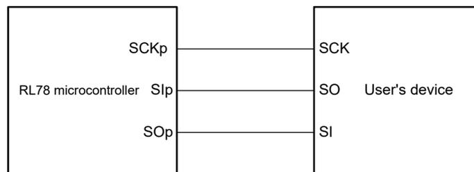
**CSI mode connection diagram (during communication at same potential)****(Slave transmission of slave select input function (CSI00))**
