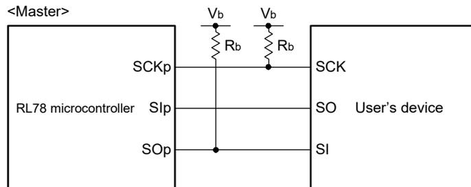
**Remark 1.**  $R_b$  [ $\Omega$ ]: Communication line (SCKp, SOp) pull-up resistance,  $C_b$  [F]: Communication line (SCKp, SOp) load capacitance,  $V_b$  [V]: Communication line voltage
