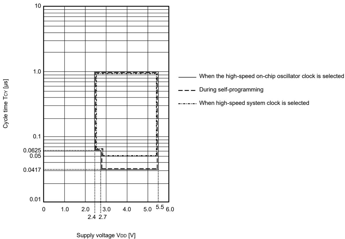
T<sub>CY</sub> vs V<sub>DD</sub> (LS (low-speed main) mode)
