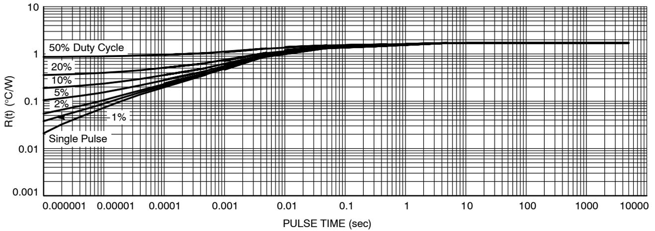
Figure 13. Thermal Characteristics
