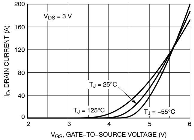
Figure 2. Transfer Characteristics
