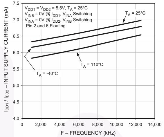
**Fig. 11b Typical  $I_{DD1}/I_{DD2}$  Supply Current vs. Frequency**
