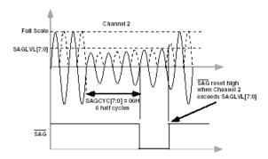
The 12-bit SAGLVL register contains the amplitude that the voltage channel must fall below before sag event occurs. The sag threshold is the number of half line cycles below which the voltage channel must remain before a sag condition occurs. Each LSB of the SAGCYC register corresponds to one half line cycle period. The default value is 0xFF(HEX). At 50Hz, the maximum sag cycle time is 2.55 seconds.
