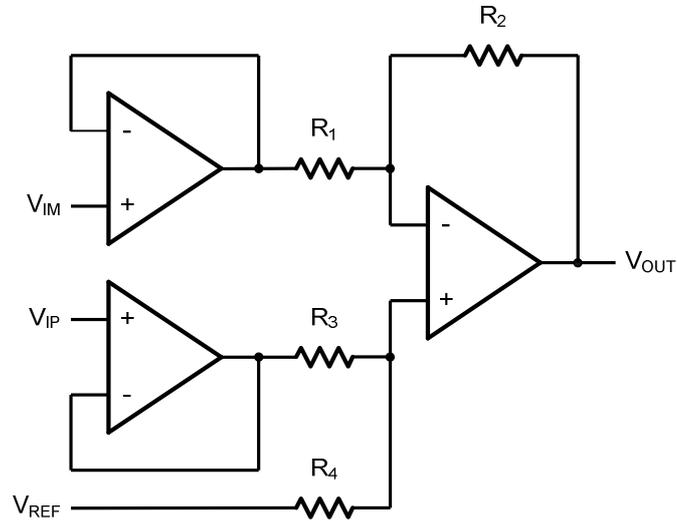
Figure 6. Instrument Amplifier
