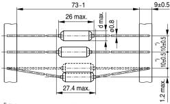
\*) Tolerance over 10 spacings ±2 mm
