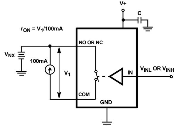
FIGURE 5.  $r_{ON}$  TEST CIRCUIT
