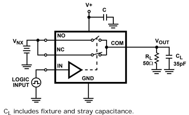
$C_L$  includes fixture and stray capacitance.
