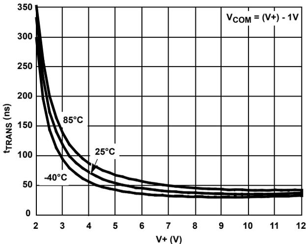
FIGURE 14. ADDRESS TRANS TIME vs SUPPLY VOLTAGE
