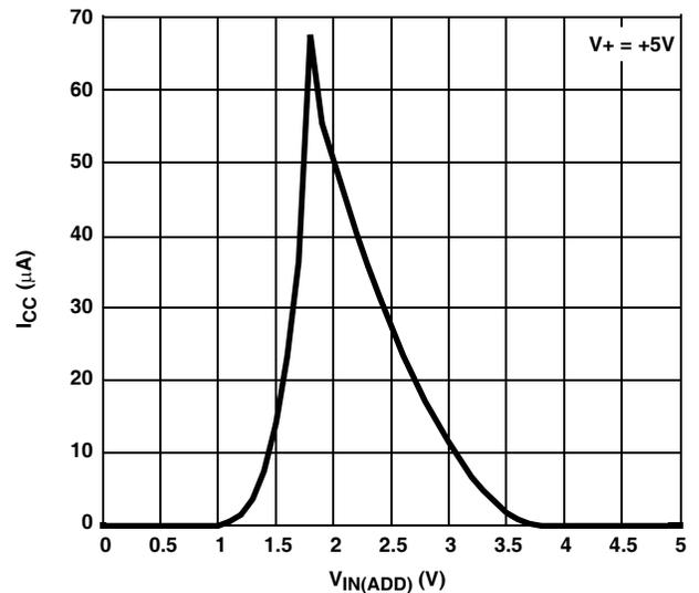
FIGURE 11. SUPPLY CURRENT vs DIGITAL ADDRESS INPUT VOLTAGE
