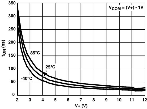
FIGURE 12. TURN - ON TIME vs SUPPLY VOLTAGE
