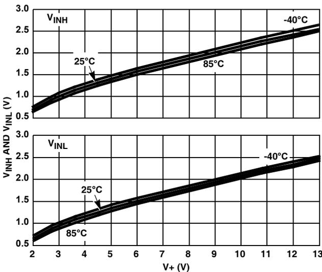
FIGURE 10. DIGITAL SWITCHING POINT vs SUPPLY VOLTAGE
