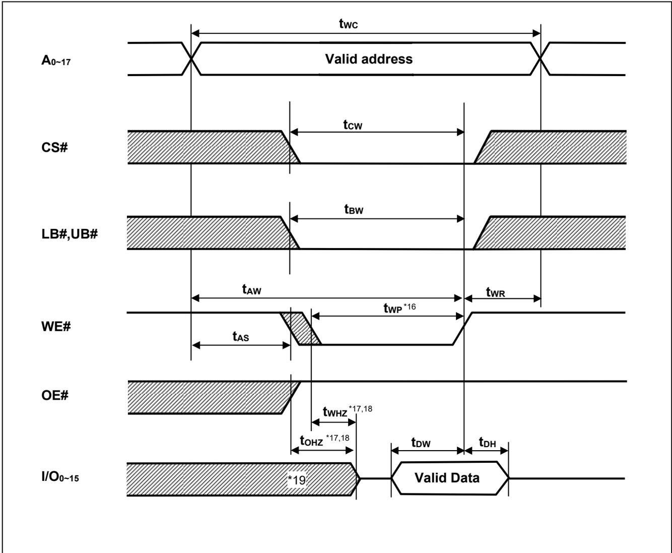
Note 16.  $t_{WP}$  is the interval between write start and write end.
