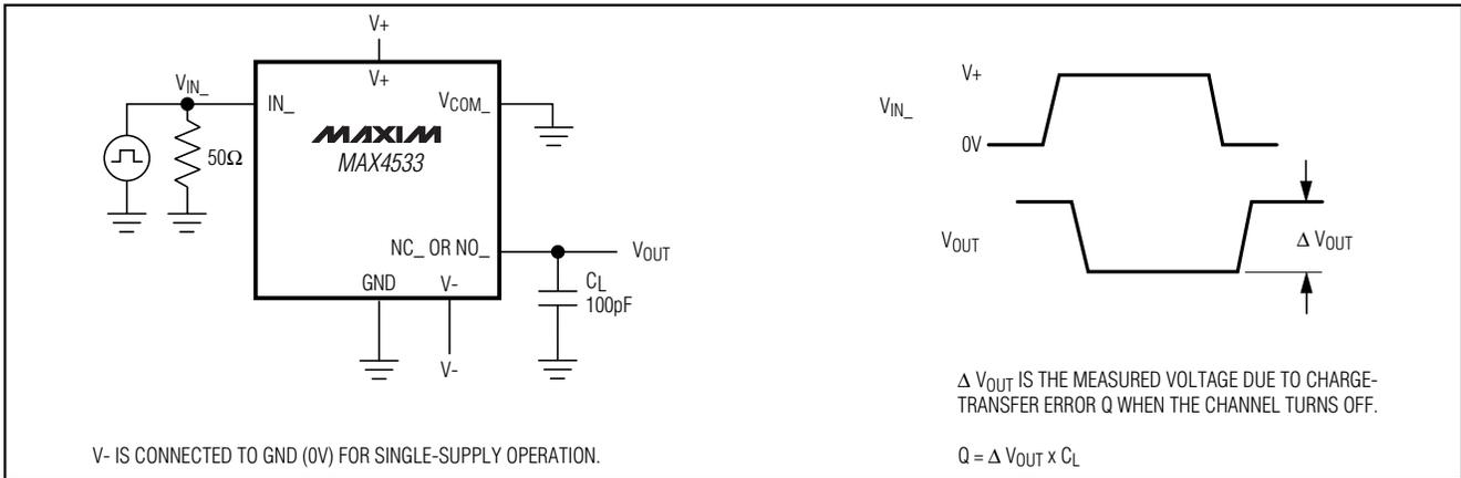
Figure 4. Charge Injection
