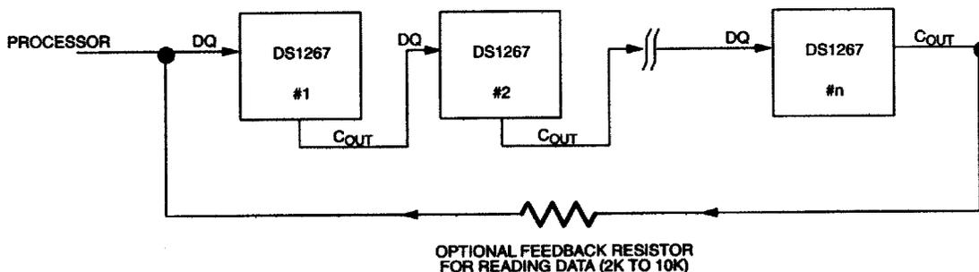
The  $C_{OUT}$  output of the DS1267B can be used to drive the DQ input of another DS1267B. When connecting multiple devices, the total number of bits transmitted is always 17 times the number of DS1267Bs in the daisy chain.
