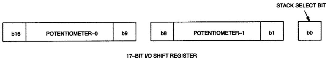
Transmission of data always begins with the stack select bit followed by the potentiometer-1 wiper position value and lastly the potentiometer-0 wiper position value.
