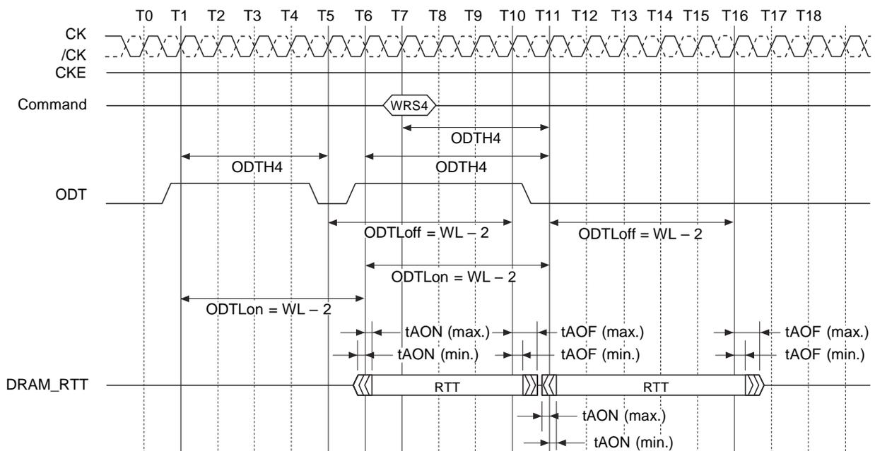
**Synchronous ODT Timing Examples (2)\*: BC4, WL = 7**
