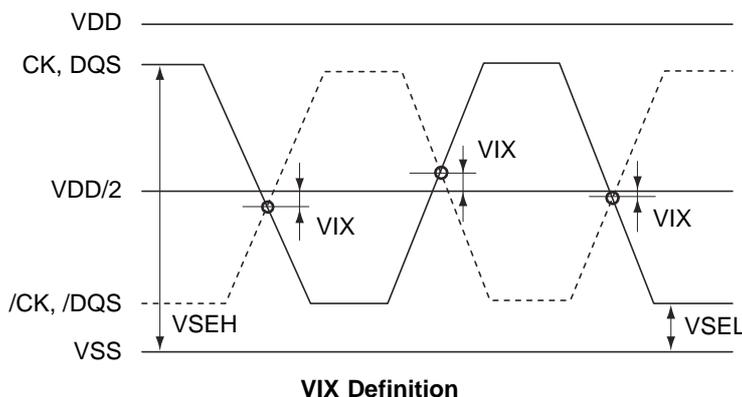
**[Cross point voltage for differential input signals (CK, DQS)]**
