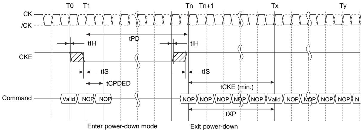
Note: Valid command at T0 is ACT, NOP, DESL or precharge with still one bank remaining open after completion of precharge command.
