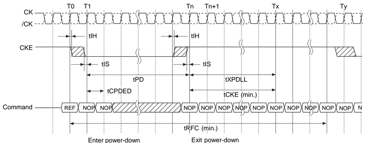
Note: \* Synchronous ODT Timing starts at the end of  $t_{XPDLL}$  (min.)
