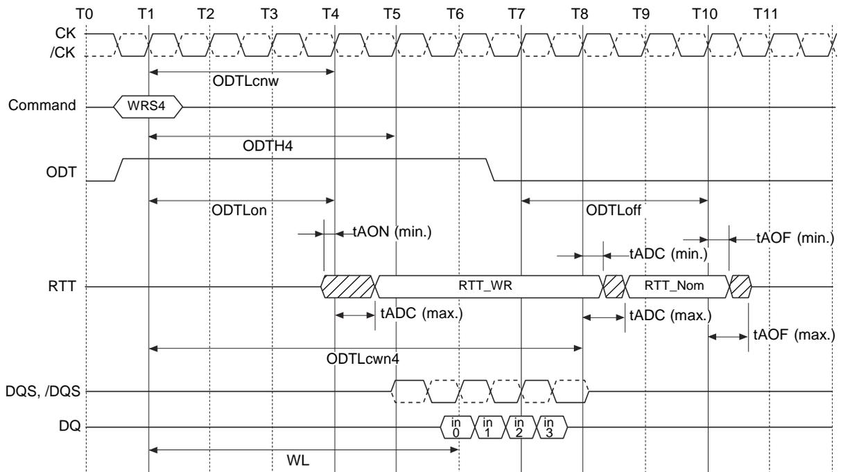
**Dynamic ODT\*: Behavior with ODT Pin Being Asserted Together with Write Command for a Duration of 6 Clock Cycles, Example for BC4 (via MRS or OTF), AL = 0, CWL = 5.**
