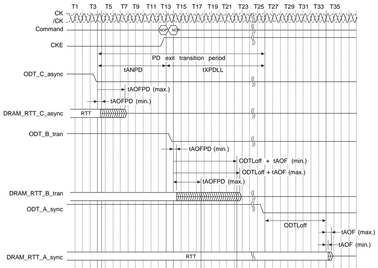
**Asynchronous to Synchronous Transition during Precharge Power-Down (with DLL Frozen) Exit**
