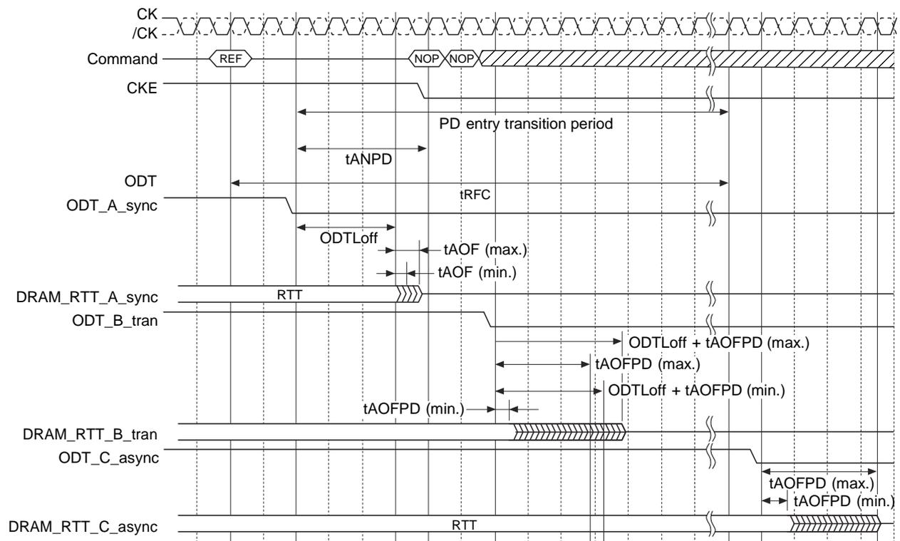
**Synchronous to Asynchronous Transition During Precharge Power-Down (with DLL Frozen) Entry**
