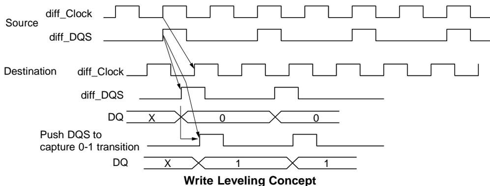
DQS, /DQS driven by the controller during leveling mode must be terminated by the DRAM, based on the ranks populated. Similarly, the DQ bus driven by the DRAM must also be terminated at the controller.
