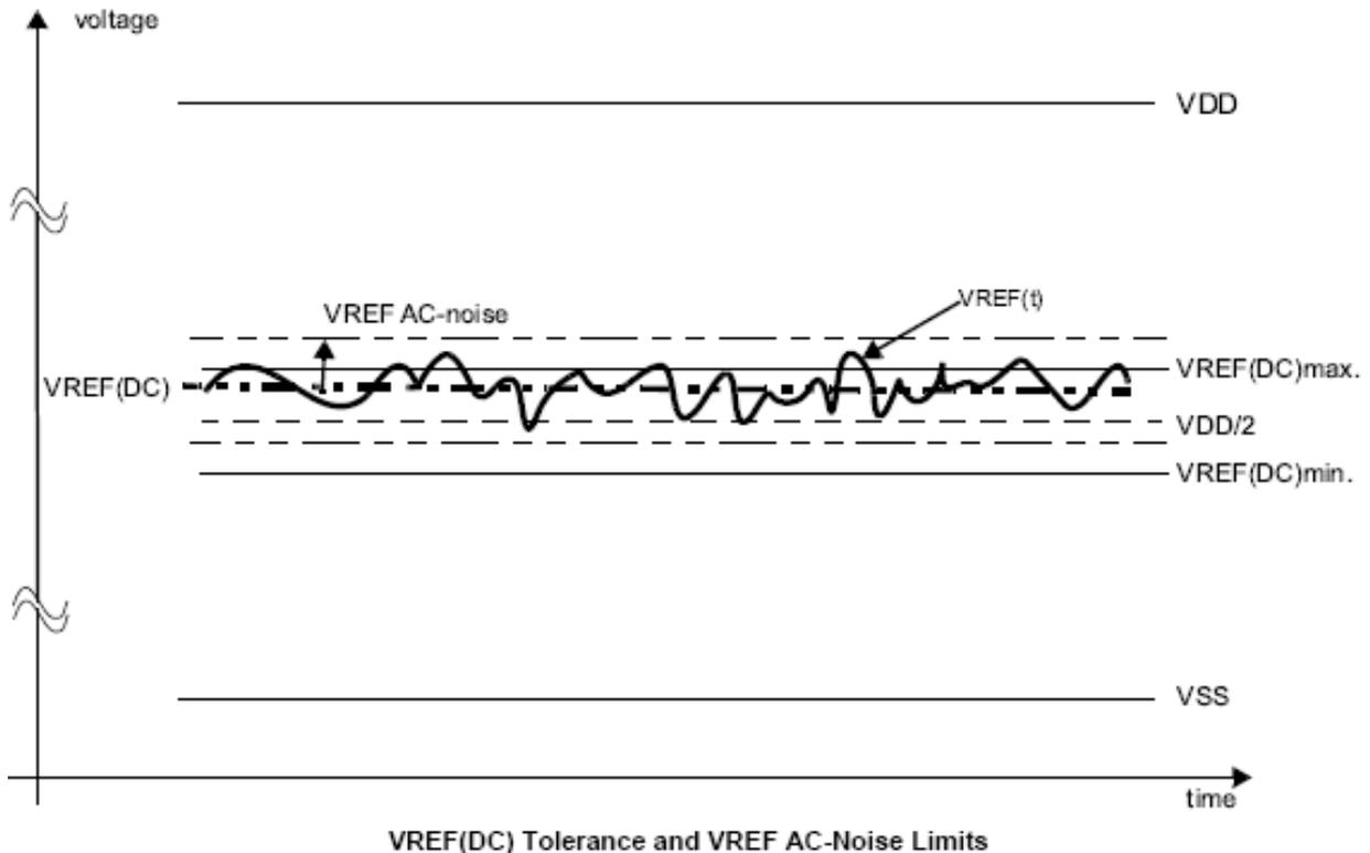
The voltage levels for setup and hold time measurements  $V_{IH}(AC)$ ,  $V_{IH}(DC)$ ,  $V_{IL}(AC)$  and  $V_{IL}(DC)$  are dependent on VREF.
