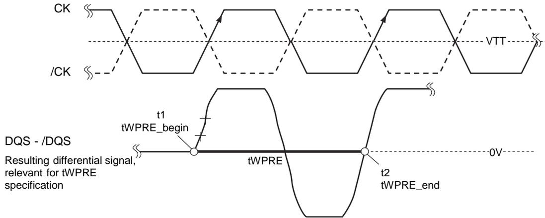
**Method for Calculating tWPRE Transitions and Endpoints**
