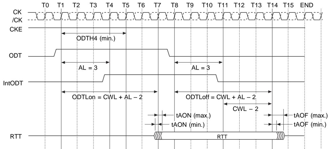
**Synchronous ODT Timing Examples (1): AL=3, CWL = 5;**
