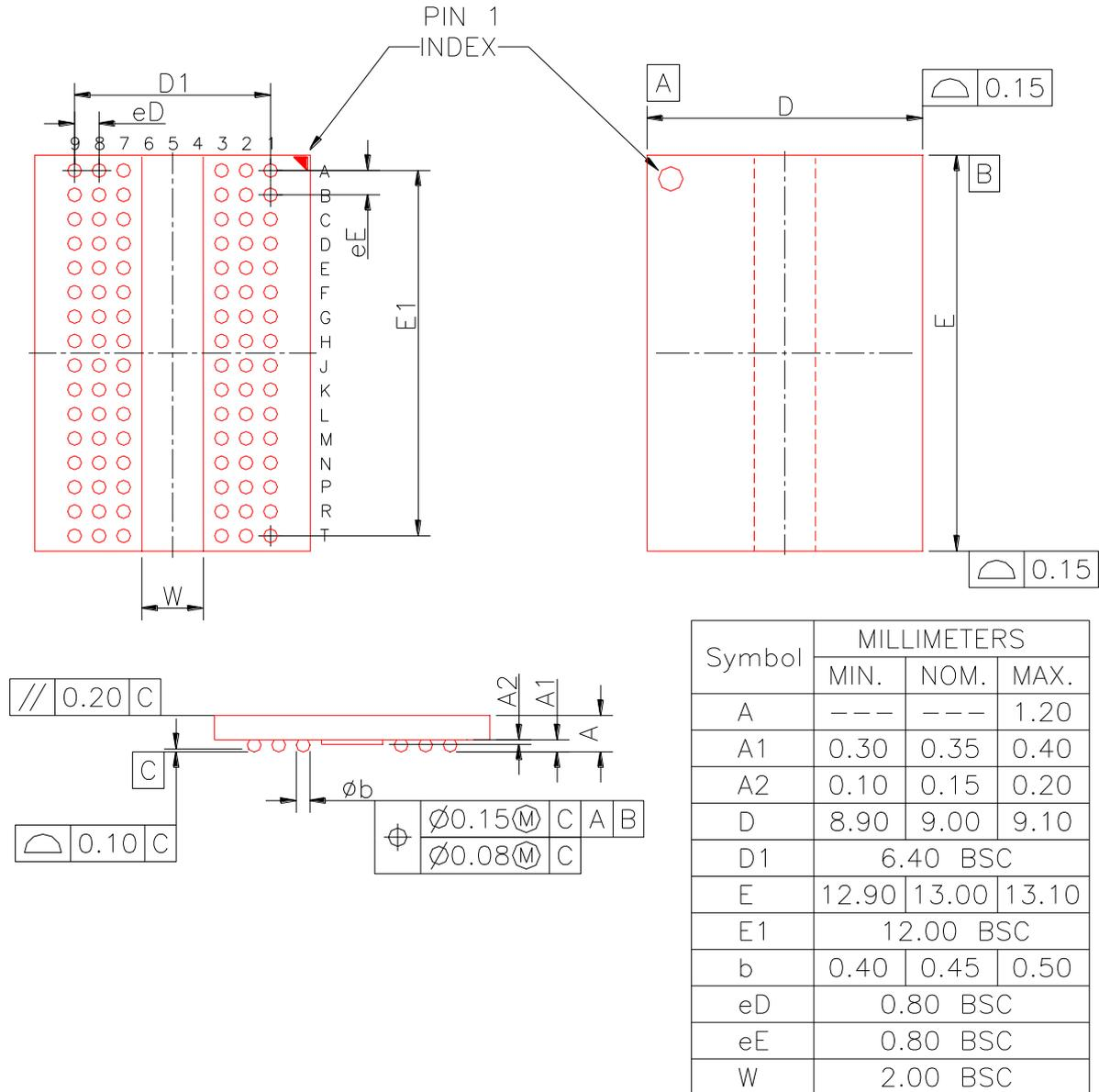
Note: The pin 1 index at bottom side is No Connection.
