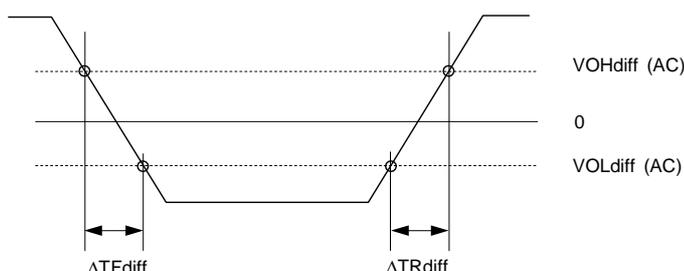
$$\text{Falling slew} = \frac{VOHdiff(AC) - VOLdiff(AC)}{\Delta TFdiff} \quad \text{Rising slew} = \frac{VOHdiff(AC) - VOLdiff(AC)}{\Delta TRdiff}$$
