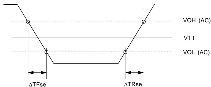
$$\text{Falling slew} = \frac{VOH (AC) - VOL (AC)}{\Delta TFse}$$
