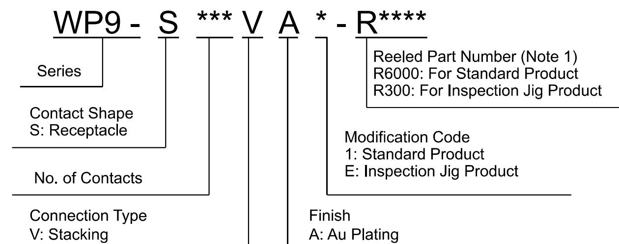
Note 1) An embossed tape reel contains 6,000 pieces of standard product, or 300 pieces of inspection jig product. Please contact us for details on embossed tape specifications.
