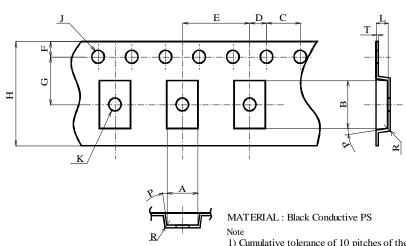
1) Cumulative tolerance of 10 pitches of the sprocket hole is  $40.0 \pm 0.2 \, \text{mm}$
