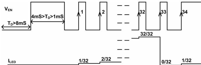
**Figure 4. Single Wire Dimming Signal on EN**
