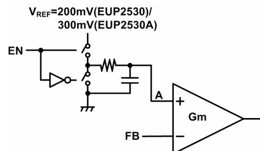
Figure 3. Block Diagram of Programmable FB Voltage Using PWM Signal
