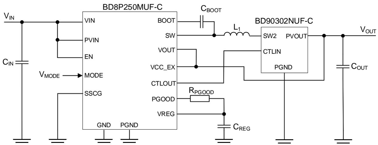
Figure 1. Application Circuit
