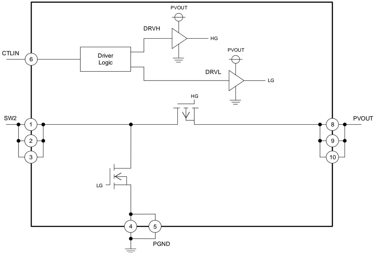
Figure 3. Block Diagram
