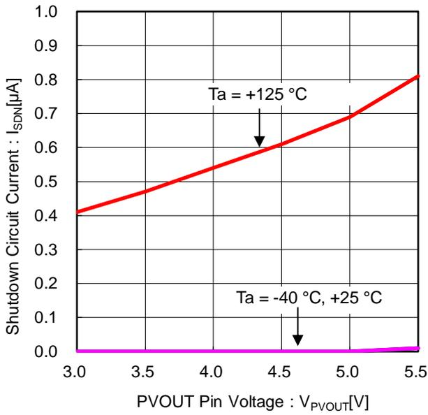
Figure 6. Shutdown Circuit Current vs PVOUT Pin Voltage
