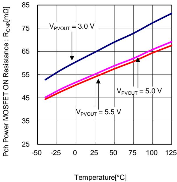
Figure 6. Pch Power MOSFET ON Resistance vs Temperature
