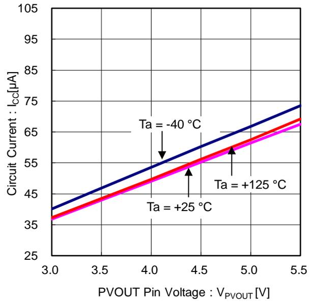
Figure 7. Circuit Current vs PVOUT Pin Voltage
