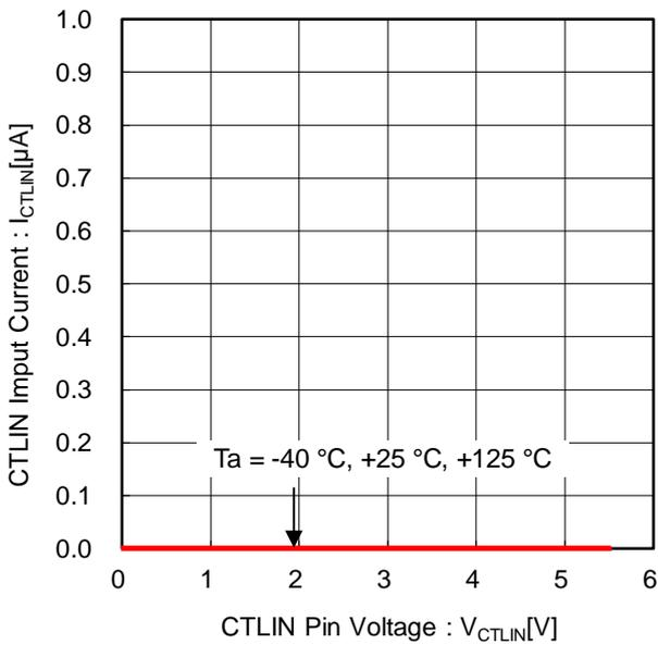
Figure 8. CTLIN Input Current vs CTLIN Pin Voltage
