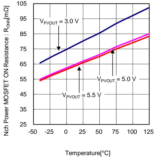
Figure 7. Nch Power MOSFET ON Resistance vs Temperature
