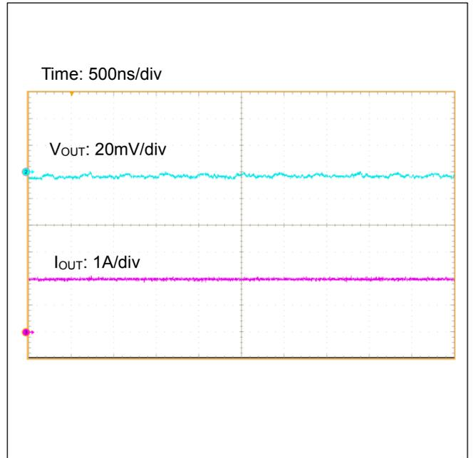
Figure 55. Output Ripple Voltage ( $I_{OUT}=2A$ )
