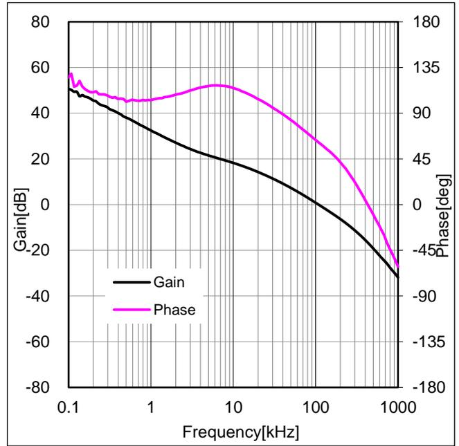
Figure 58. Frequency Characteristics (I<sub>OUT</sub>=2A)
