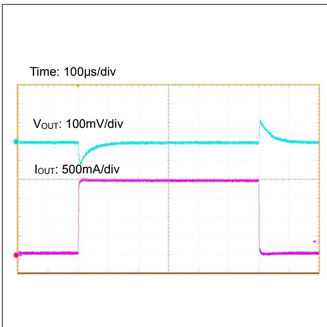
Figure 44. Load Transient Response ( $I_{OUT}=0A \leftrightarrow 2A$ )
