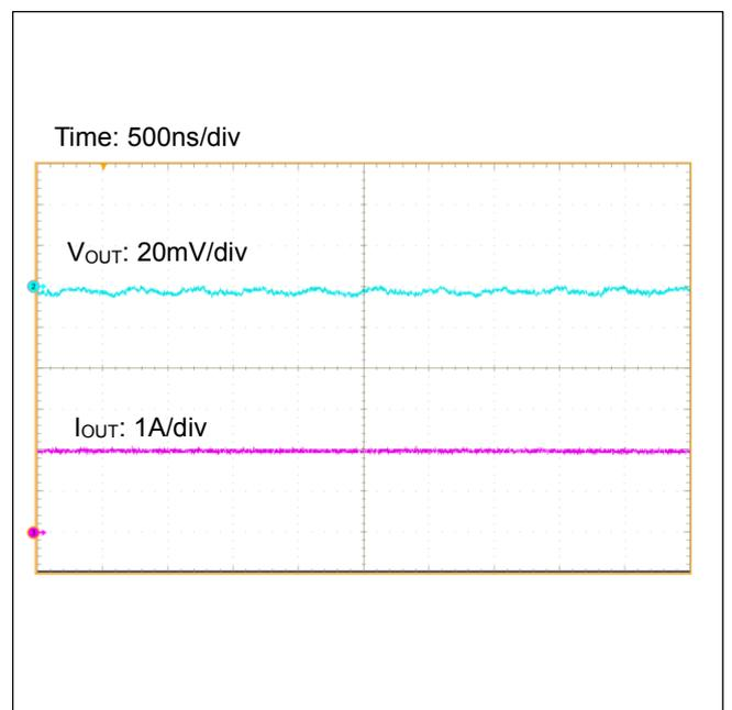
Figure 65. Output Ripple Voltage (I<sub>out</sub>=2A)
