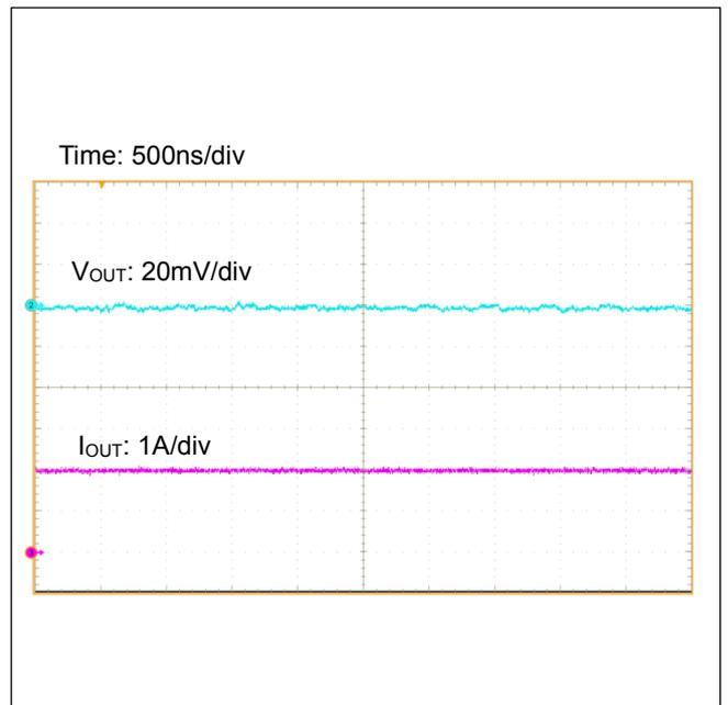
Figure 60. Output Ripple Voltage (I<sub>OUT</sub>=2A)
