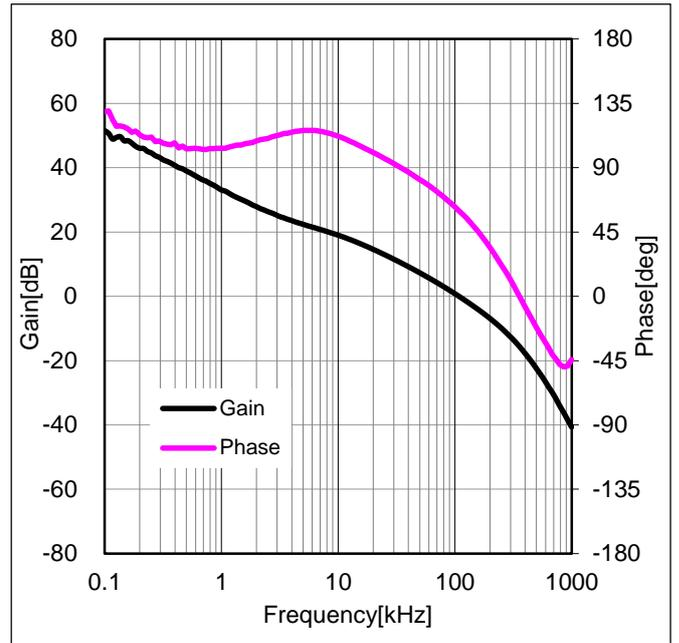
Figure 63. Frequency Characteristics (I<sub>out</sub>=2A)
