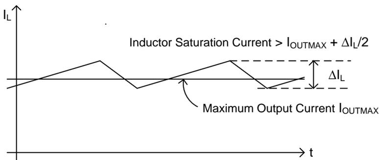
Figure 36. Waveform of Current Through Inductor
