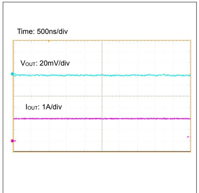
Figure 50. Output Ripple Voltage (I<sub>OUT</sub>=2A)
