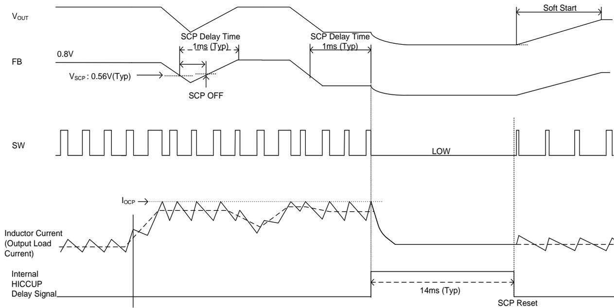
Figure 31. Short Circuit Protection (SCP) Timing Chart
