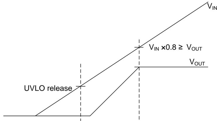
Figure 40. Input Voltage Startup Time
