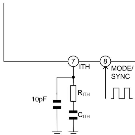
Figure 27. Recommended Circuit When Using External Synchronization Function
