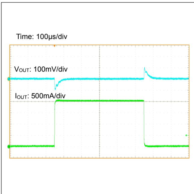
Figure 64. Load Transient Response (I<sub>out</sub>=0A↔2A)
