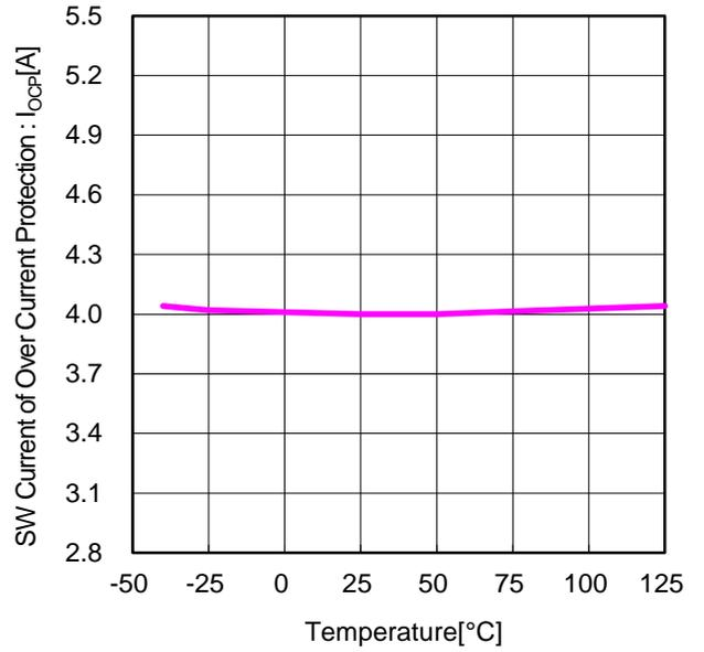
Figure 21 SW Current of Over Current Protection vs Temperature
