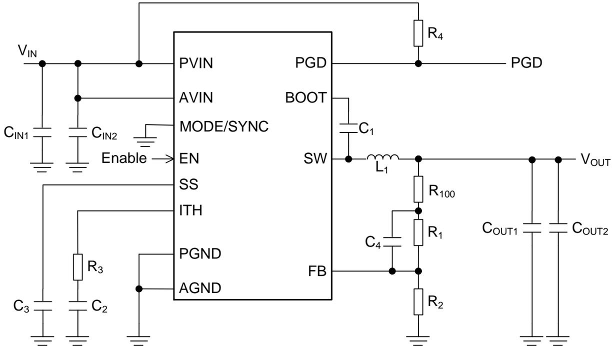
Figure 66. Reference Circuit 6
