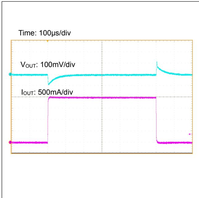
Figure 54. Load Transient Response ( $I_{OUT}=0A \leftrightarrow 2A$ )
