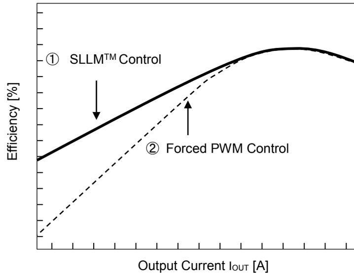
Figure 28. Efficiency (SLLM™ Control and Forced PWM Control)
