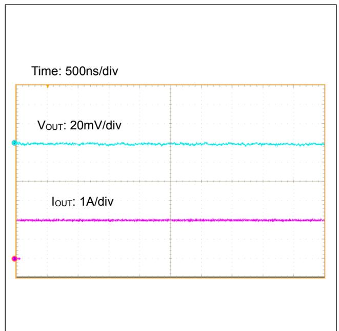
Figure 45. Output Ripple Voltage ( $I_{OUT}=2A$ )
