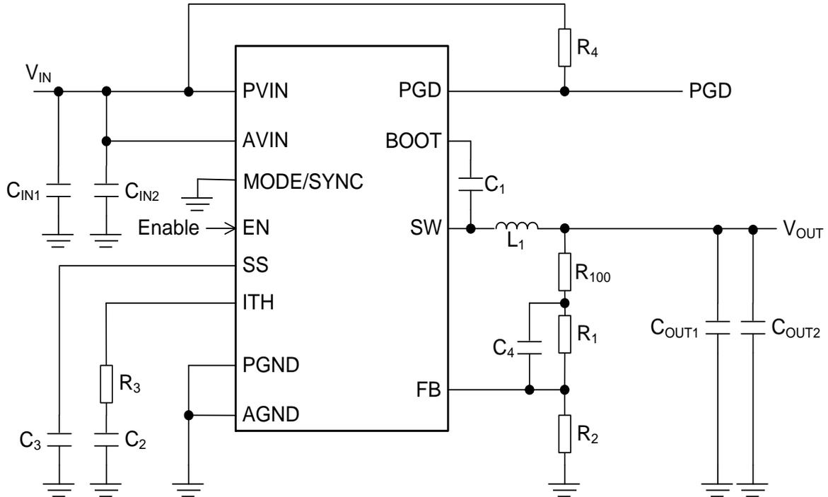
Figure 41. Reference Circuit 1
