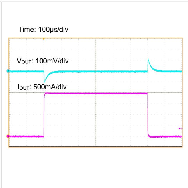
Figure 69. Load Transient Response ( $I_{OUT}=0A \leftrightarrow 2A$ )
