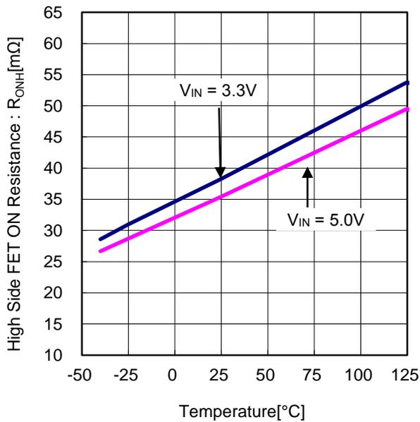
Figure 14. High Side FET ON Resistance vs Temperature
