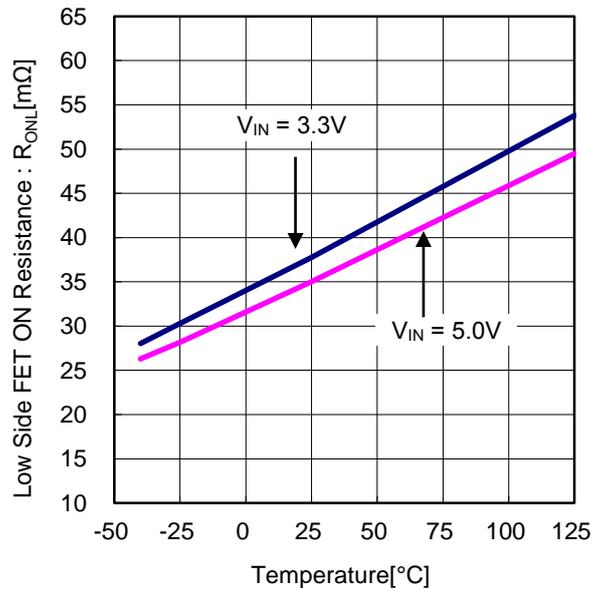
Figure 15. Low Side FET ON Resistance vs Temperature
