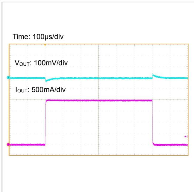
Figure 49. Load Transient Response (I<sub>OUT</sub>=0A↔2A)
