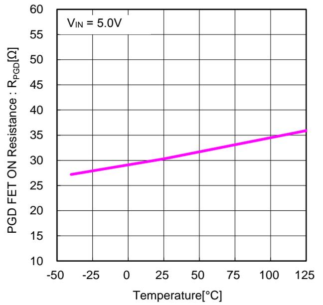
Figure 17. PGD FET ON Resistance vs Temperature
