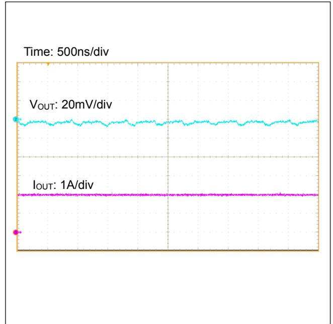
Figure 70. Output Ripple Voltage ( $I_{OUT}=2A$ )
