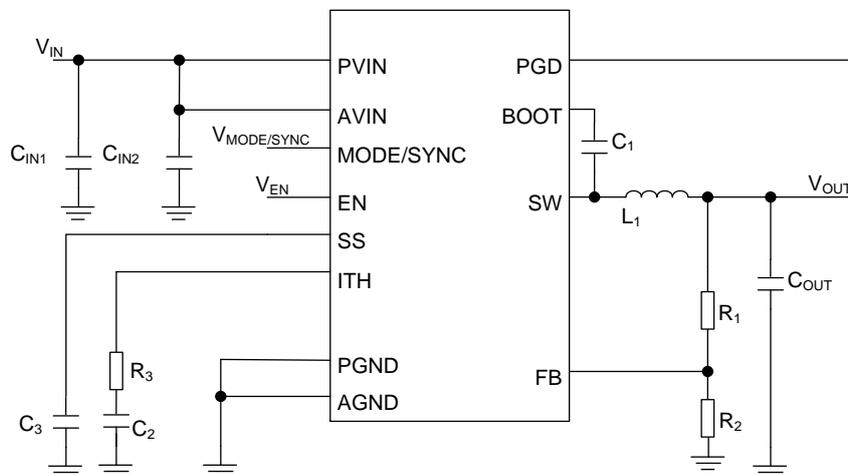
Figure 1. Application Circuit
