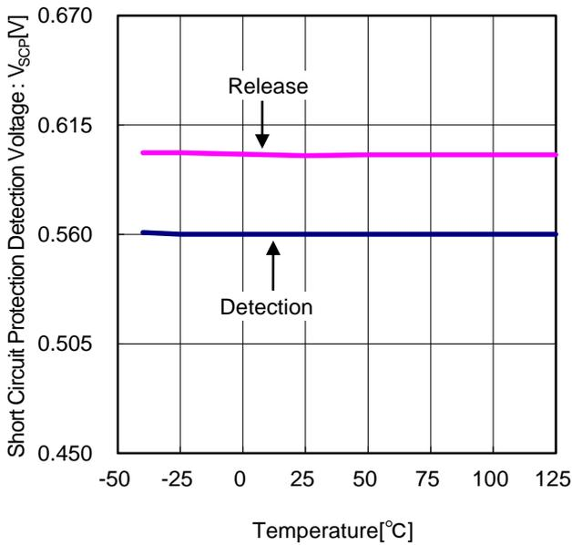
Figure 22. Short Circuit Protection Detection Voltage vs Temperature
