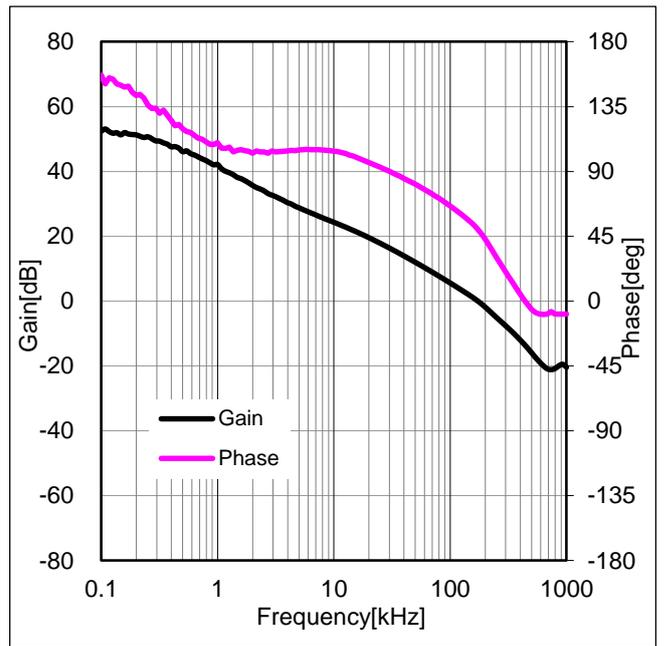
Figure 48. Frequency Characteristic (I<sub>OUT</sub>=2A)
