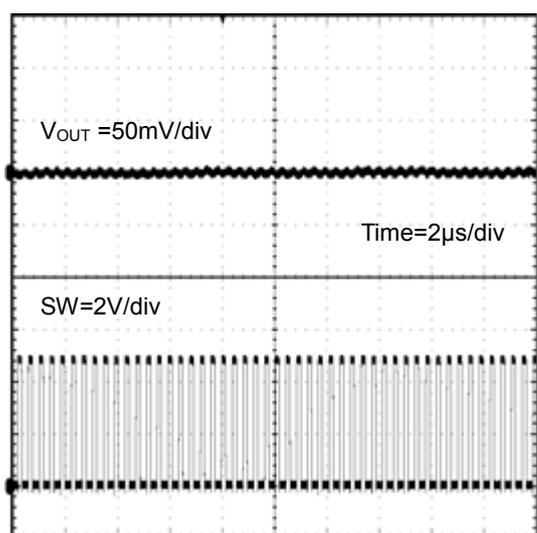
Figure 30. SW Waveform (Forced PWM Control)
