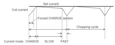
Charge mode continues until ICOIL  $\geq$  IREF. After that the IC switches to SLOW DECAY mode and then switches to FAST DECAY mode for the last about 1 $\mu$ s.
