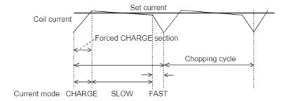
The IC switches to SLOW DECAY after Blanking section, and then switches to FAST DECAY mode for the last about  $1\mu s$ .
