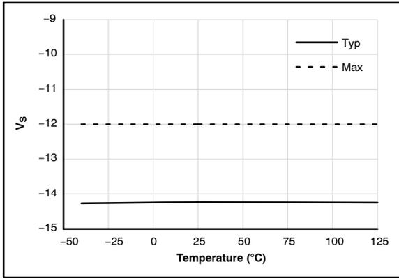
Figure 28. Allowable Negative  $V_S$  Voltage vs. Temperature
