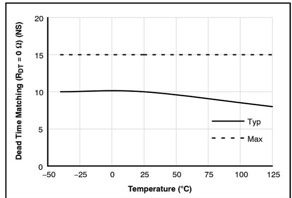
Figure 9. Dead Time Matching ( $R_{DT} = 0 \Omega$ ) vs. Temperature
