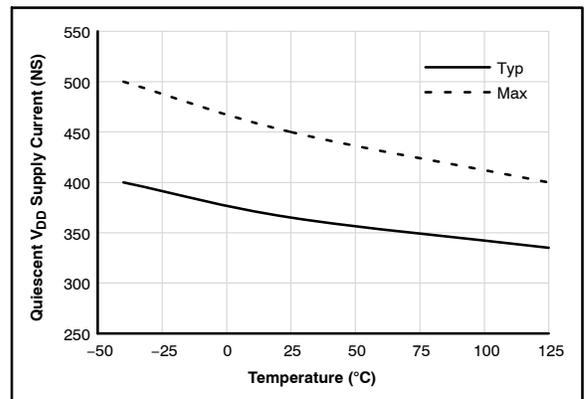
Figure 15. Quiescent  $V_{DD}$  Supply Current vs. Temperature
