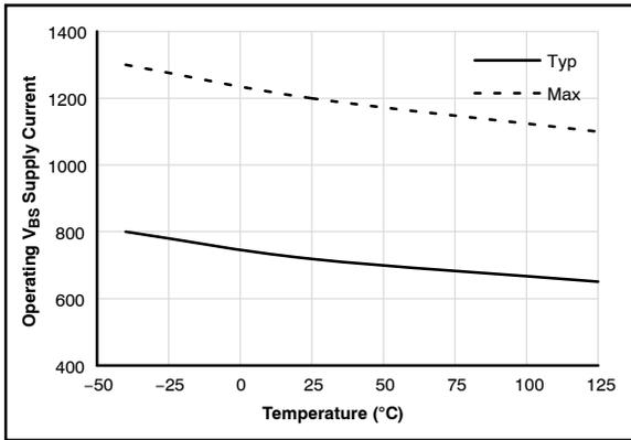
Figure 18. Operating  $V_{BS}$  Supply Current vs. Temperature
