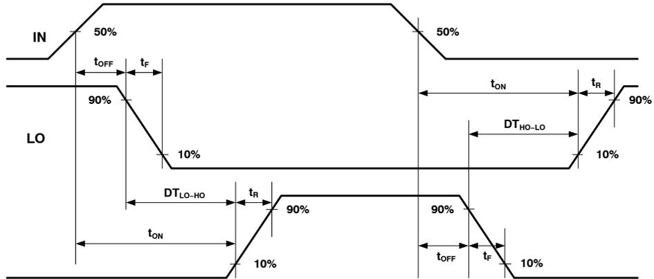
Figure 33. Switching Time and Dead-Time Waveform Definition
