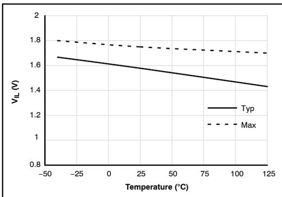
Figure 26. Logic LOW Input Voltage vs. Temperature
