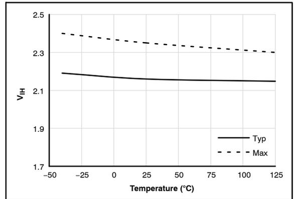
Figure 25. Logic HIGH Input Voltage vs. Temperature
