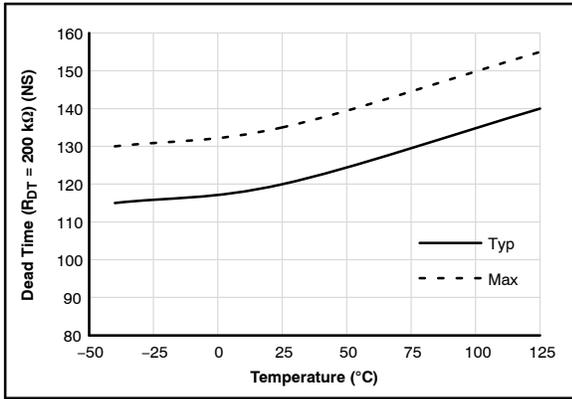
Figure 10. Dead Time ( $R_{DT} = 200\text{ k}\Omega$ ) vs. Temperature
