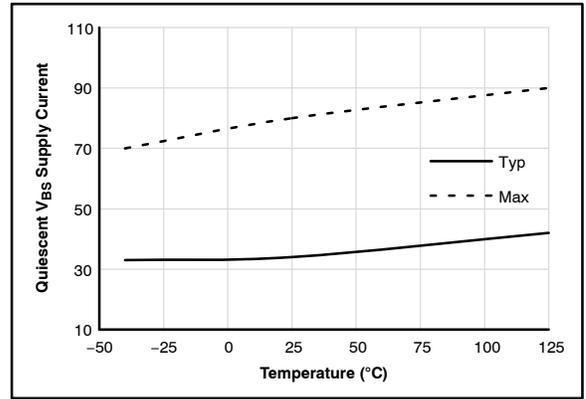
Figure 17. Quiescent  $V_{BS}$  Supply Current vs. Temperature
