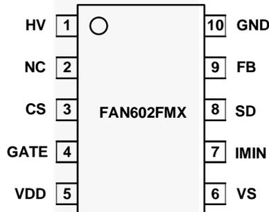
Figure 4. Pin Assignment
