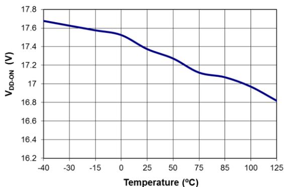
Figure 5. Turn-On Threshold Voltage (V<sub>DD-ON</sub>) vs. Temperature
