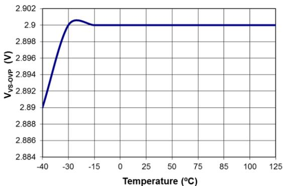
**Figure 15. Output Over-Voltage-Protection ( $V_{VS-OVP}$ ) vs. Temperature**
