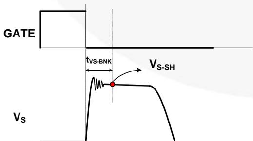
**Figure 29. Output Voltage Detection**
