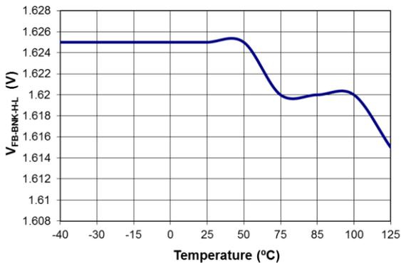
**Figure 13. Frequency Jumping point ( $V_{FB-BNK-H-L}$ ) vs. Temperature**
