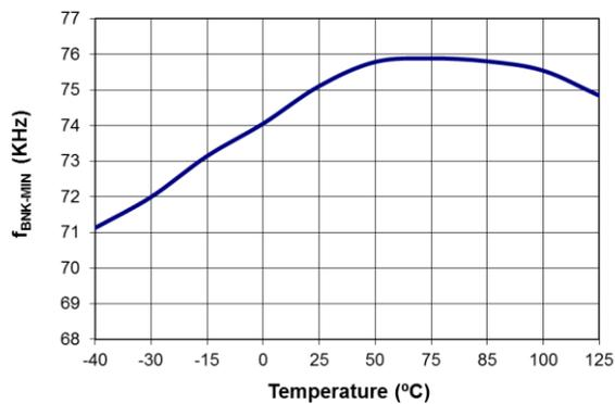
Figure 10. Minimum Blanking Frequency (f<sub>BNK-MIN</sub>) vs. Temperature
