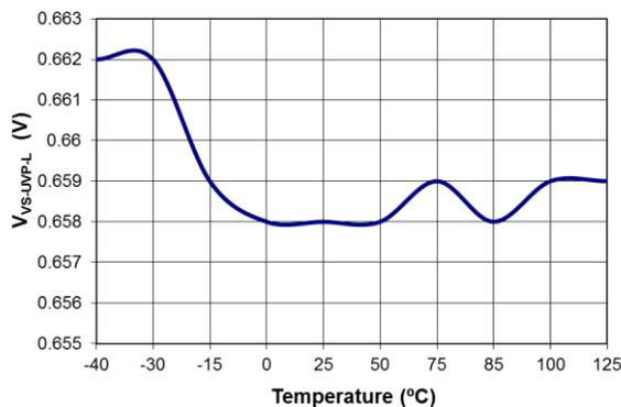
**Figure 16. Output Under-Voltage Protection ( $V_{VS-UVP-L}$ ) vs. Temperature**
