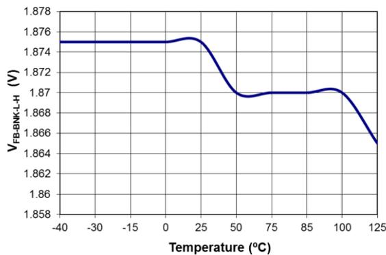
**Figure 12. Frequency Jumping point ( $V_{FB-BNK-L-H}$ ) vs. Temperature**
