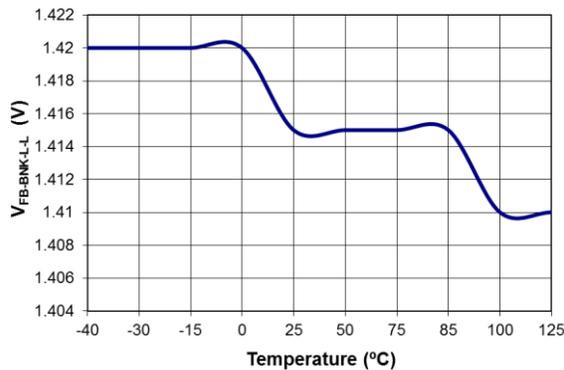
**Figure 14. Frequency Jumping point ( $V_{FB-BNK-L-L}$ ) vs. Temperature**
