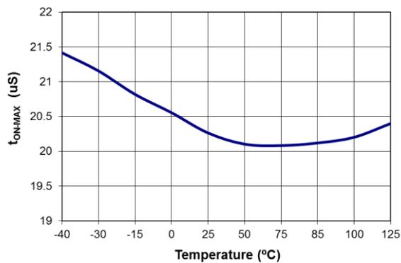
Figure 22. Maximum On Time ( $t_{ON-MAX}$ ) vs. Temperature
