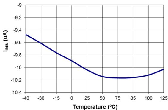
Figure 19. IMIN Pin Current ( $I_{IMIN}$ ) vs. Temperature
