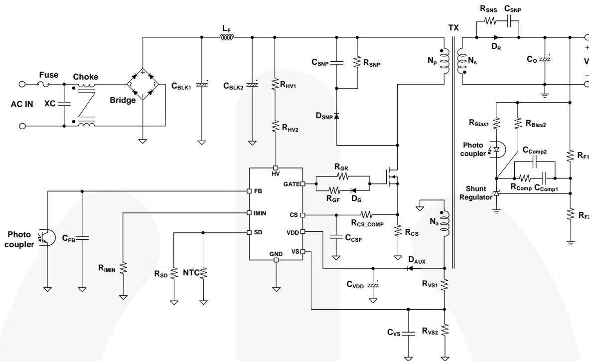
Figure 1. FAN602F Typical Application
