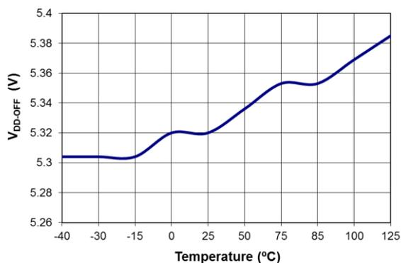
Figure 6. Turn-Off Threshold Voltage (V<sub>DD-OFF</sub>) vs. Temperature
