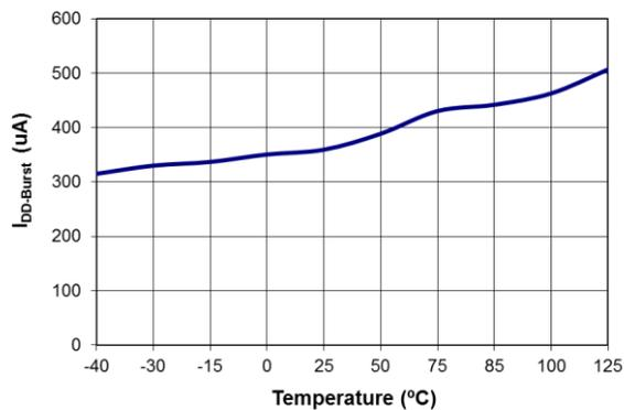
Figure 8. Burst-Mode Operating Supply Current (I<sub>DD-Burst</sub>) vs. Temperature
