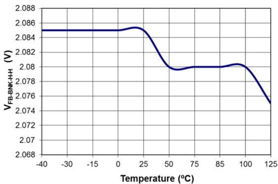
**Figure 11. Frequency Jumping point ( $V_{FB-BNK-H-H}$ ) vs. Temperature**
