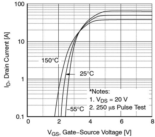
**Figure 2. Transfer Characteristics**
