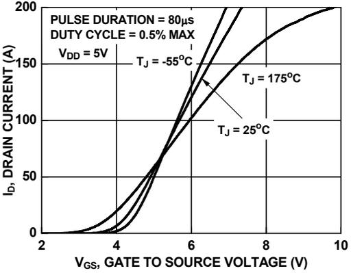
**Figure 7. Transfer Characteristics**
