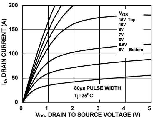
**Figure 9. Saturation Characteristics**
