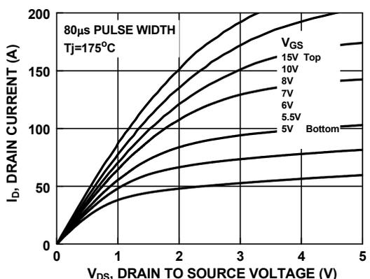
**Figure 10. Saturation Characteristics**
