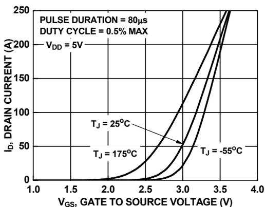
Figure 7. Transfer Characteristics
