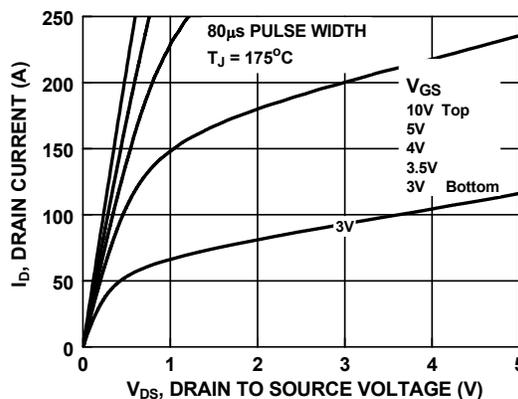
Figure 10. Saturation Characteristics
