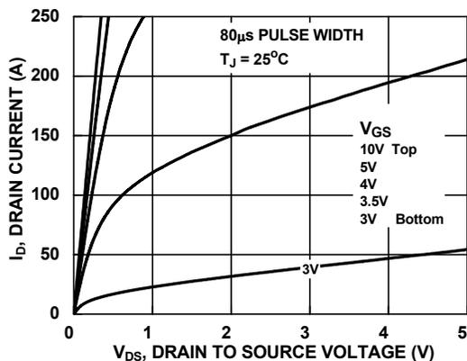
Figure 9. Saturation Characteristics
