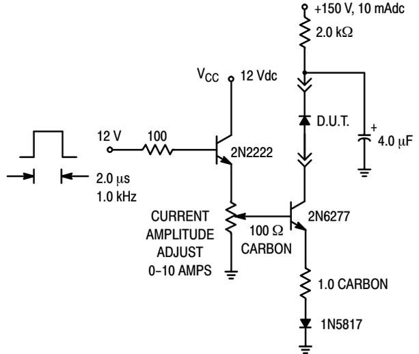
Figure 6. Test Circuit for Repetitive Reverse Current
