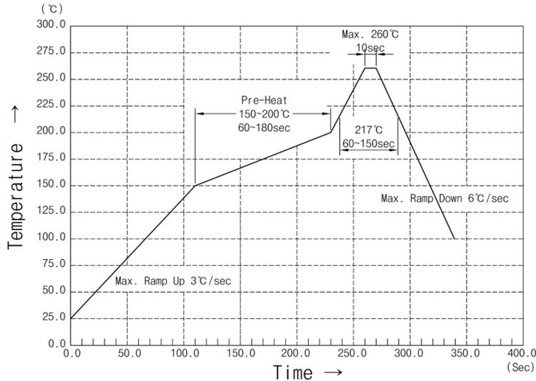
Recommended lead free reflow soldering temperature profile.
