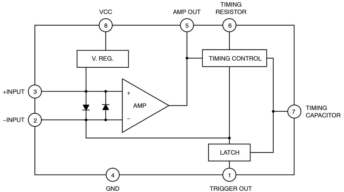
Figure 2. KA2807 Block Diagram
