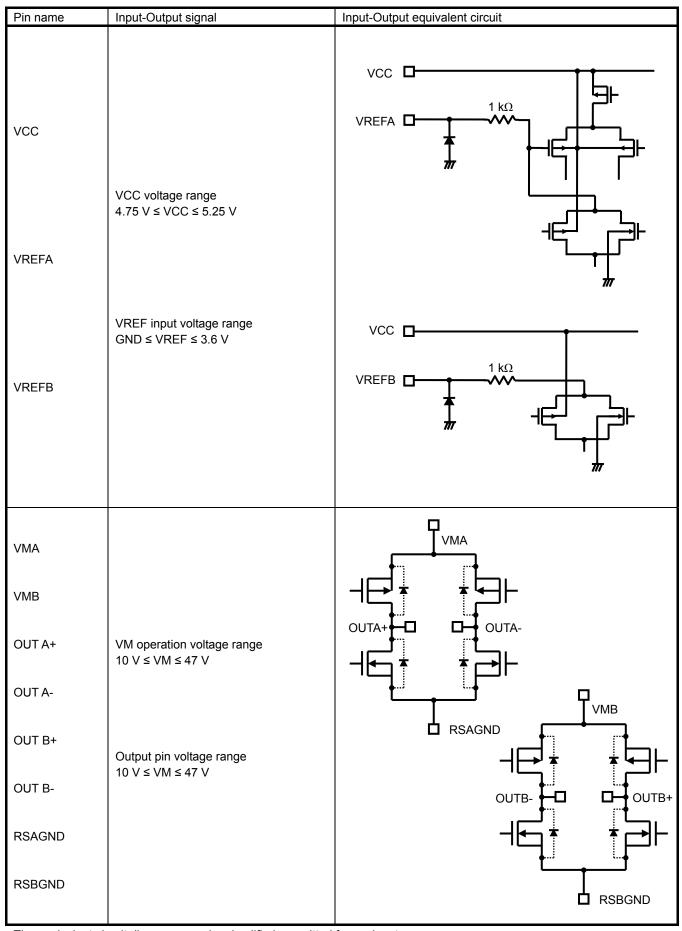
The equivalent circuit diagrams may be simplified or omitted for explanatory purposes.
