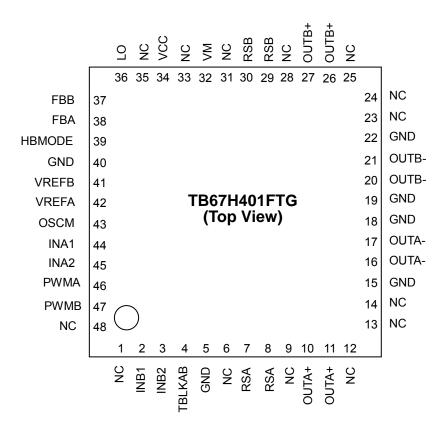
Note: Please solder the corner pad and the bottom thermal pad of the QFN package, to the GND pattern of the PCB. Note: Pin names in the above figure are in the state when HBMODE pin is low level.
