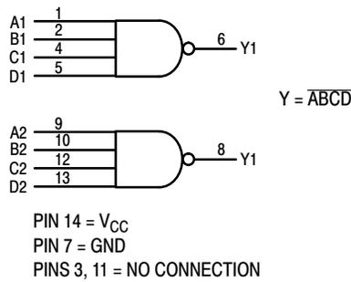
Figure 1. Logic Diagram
