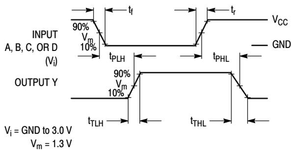
Figure 2. Switching Waveforms
